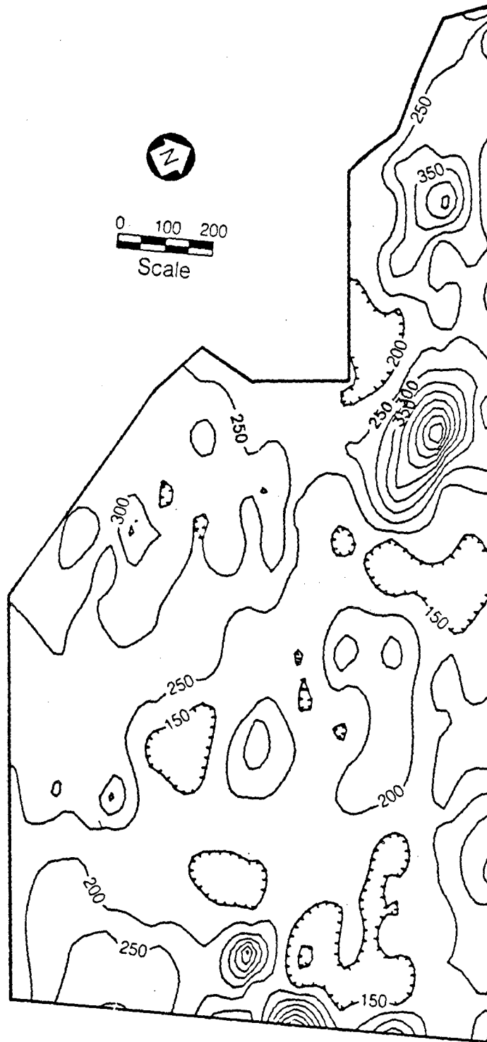
Figure 8. Isoconductivity contours for 1988 based on measurements with the Geonics EM34 with a 20-m intercoil separation. Contour interval is 50 mS/m.
