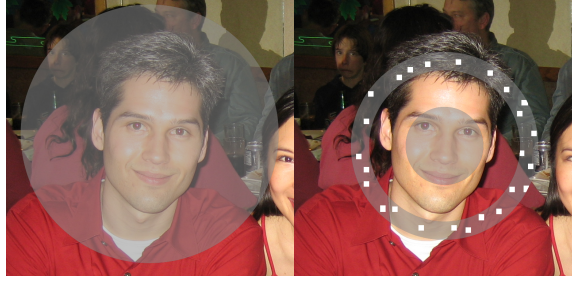
Figure 7.1. A. Circular search region with radius s (left). B. Circular region with radius r for positive examples and sampled annular region with radii q and q' for negative examples (right).
