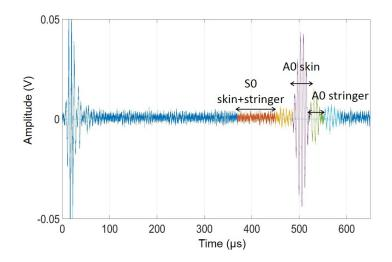
Figure 8. Typical RF waveform measured by the air-coupled pitch-catch prototype from Test Panel 3.
