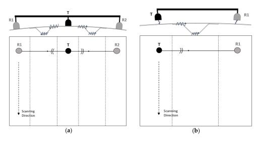
**Figure 4.** Line scanning approach for (**a**) a contact system and (**b**) a non-contact system; cross-sectional view (top drawings) and front view (bottom drawings).
