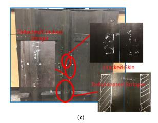
**Figure 1.** Test specimens: (a) Panel 1: five stringers, three C-frame panels with cracked skin, and a cracked stringer; (b) Panel 2: four stringers, three C-frame panels with a disbonded/detached stringer; (c) Panel 3: three stringers, two C-frame panels with cracked skin, a detached/cracked stringer, and a disbonded stringer.
