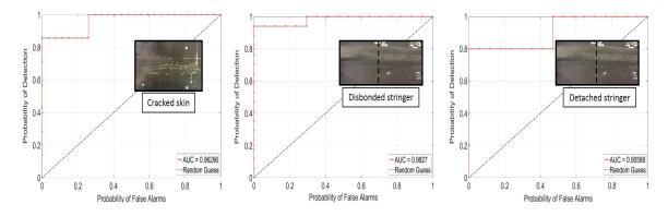
**Figure 11.** Receiver operating characteristic (ROC) curves for the contact non-destructive evaluation (NDE) technique: cracked skin, disbonded stringer, and detached stringer defects (Panel 1 and Panel 2).
