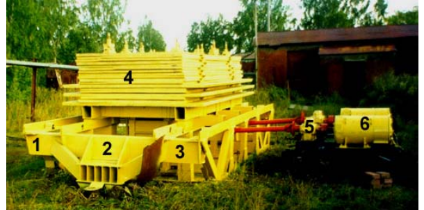
Figure 4. A view of the 40-ton vibrator. 1, 2, 3 -platform elements; 4-loading mass; 5-transmission; 6-electric motors.
