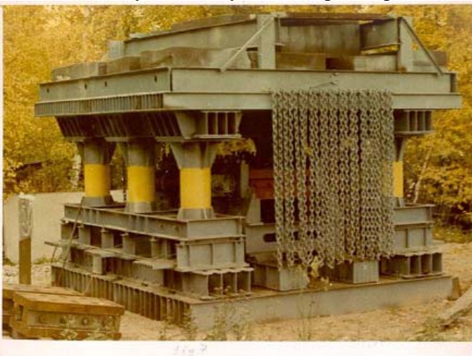
Figure 3. A view of the 100-ton vibrator.
