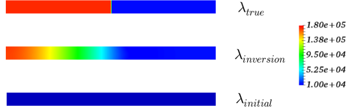
Figure 5.9: The true parameter \lambda_{true} with a discontinuity (top), reconstructed parameter field (middle) and the initial guess for Newton iterations (bottom). The true parameter \lambda_{true} is calculated by substituting E = 3 \times 10^5 , \nu = 0.3 for x \in [0, 4] and E = 2 \times 10^4 , \nu = 0.3 for x \in (4, 8] in Eq. 5.24.
