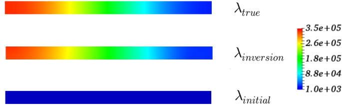
Figure 5.6: The true parameter \lambda_{true} with sinusoidal variation (top), reconstructed parameter field (middle) and the initial guess for Newton iterations (bottom).
