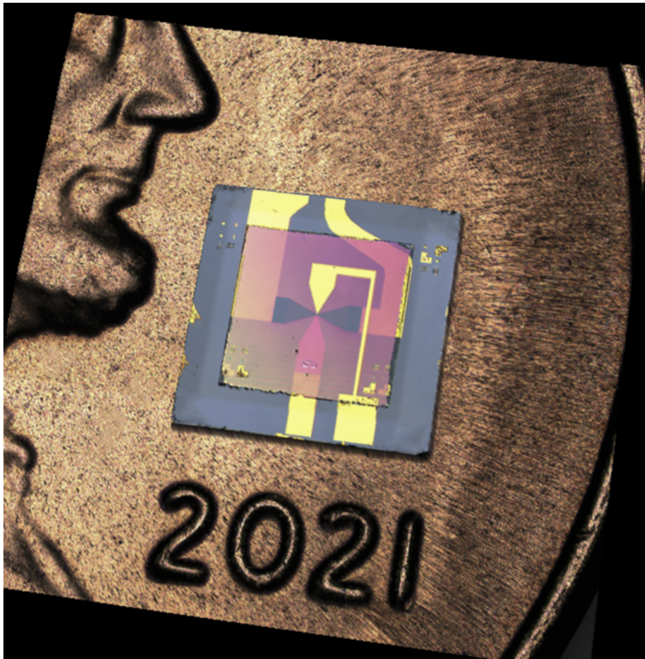
Figure 1.4: Capacitively-coupled prototype TACIT mixer on a penny (it is a real device now!) [51].
