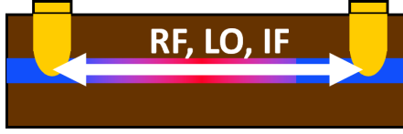
Figure 1.2: Schematic showing the two-terminal geometry of a conventional 2DEG-based HEB mixer. A planar THz antenna is integrated with the two Ohmic contacts shown in the schematic. The antenna orients the electric fields of THz RF and LO along the 2DEG plane for coupling via Joule heating in the 2DEG. The heating results in the change in the mobility of the 2DEG and results in the change in the in-plane resistance of the 2DEG. This bolometric response for the IF is coupled out by the two Ohmic contacts.
