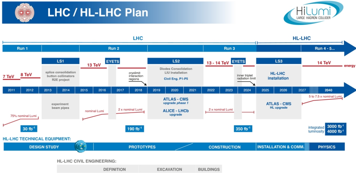
Figure 6.1: The schedule for the future LHC runs. After LS3 the luminosity will be 5 \times 10^{34} \text{ cm}^{-2} \text{ s}^{-1} . Image from [120].
