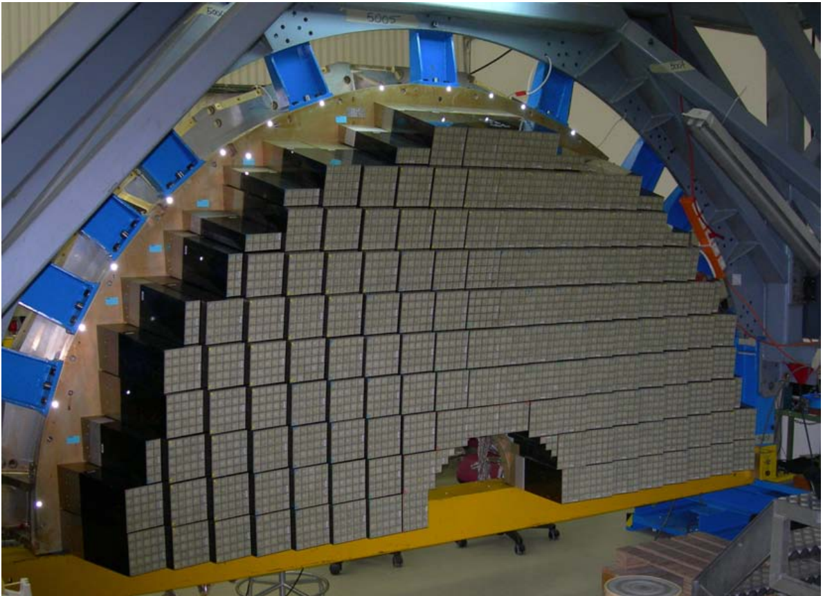
Figure 2.11: An endcap Dee. A Dee is half of one endcap. The crystals are grouped in units of 5x5 crystals called supercrystals. [53].
