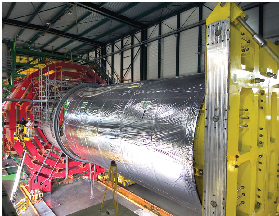
Figure 2.19: The solenoid being inserted in the cryostat barrel. [64].
