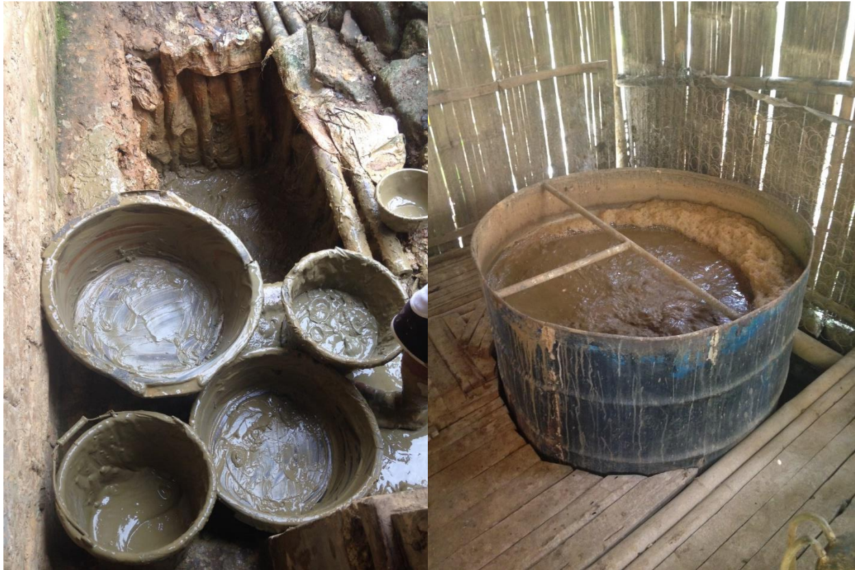
Figure 9: Left, buckets with tailings mud ( lumpur ) and, right, a cyanidation vat ( tong ) used to extract additional gold from the tailings.
