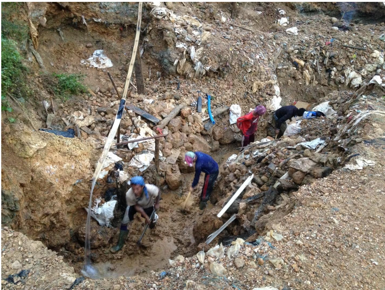
Figure 15: Miners loosening sediments with water and hoes in surface-level mining. The sediments flow down the ditch and are caught by other workers who use sluice-like boxes covered in towels.
