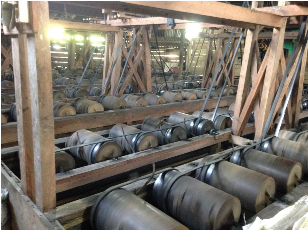
Figure 8: A very large array of gelundung (ore mills) set up in a warehouse located in a village outside of the mining concession.
