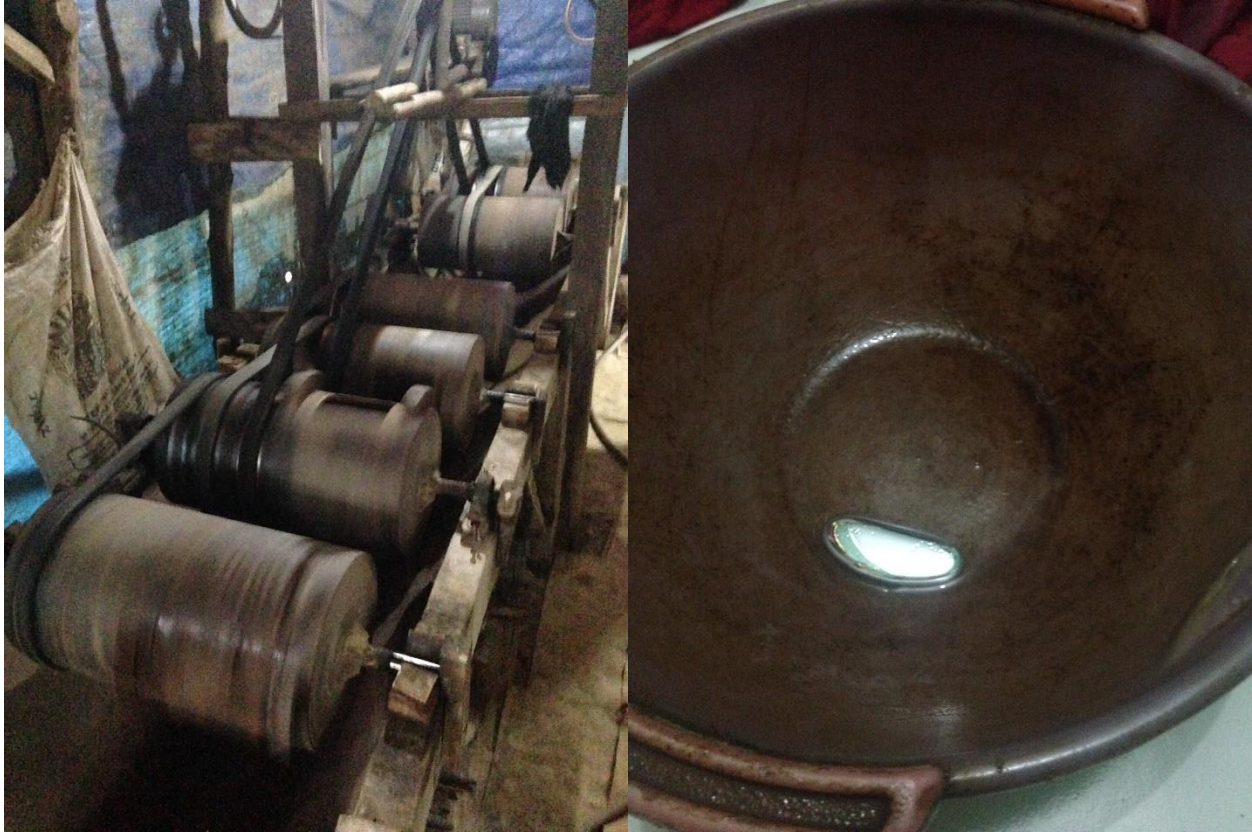
Figure 13: Left, a rotating set of gelundung. These ore mills are used to crush ore and mix it with mercury. Right, a small amount of mercury is added to each gelundung barrel, within which it will amalgamate with the gold content of the ore.
