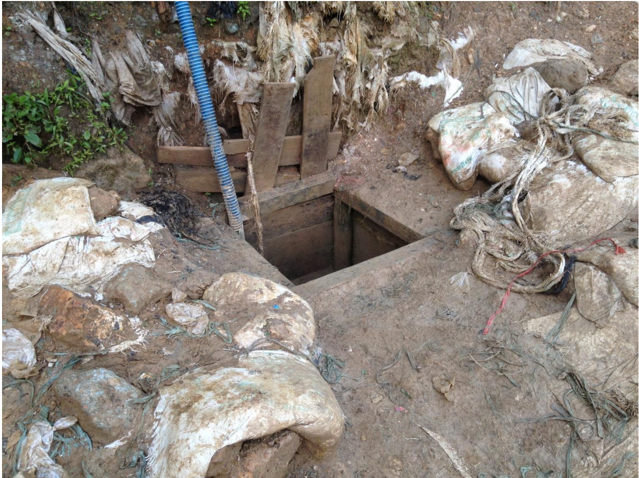
Figure 11: The primary entry point to Haji Deden's tunnel. This tunnel, with its wood-reinforced structure and hose for blowing cool air from the surface, is typical of mines that are operated by a wealthier mining boss.
