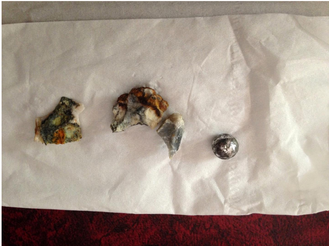
Figure 14: Two small chunks of quartz vein believed to contain gold (left and middle) and a gold-mercury amalgam ball produced through processing in a gelundung (right). The ball appears silver because the gold content is low relatively to mercury, silver, and other impurities.
