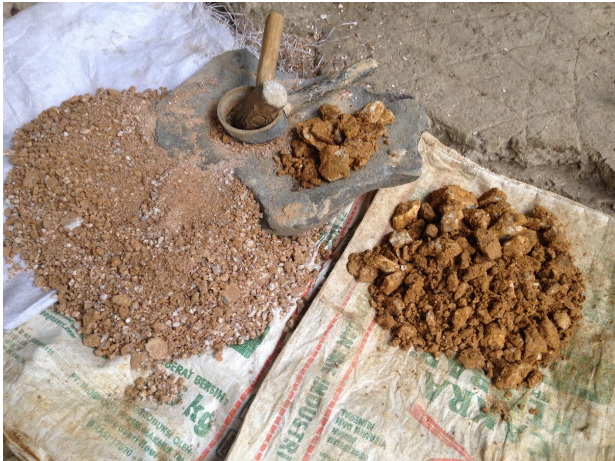
Figure 12: Laborers crush chunks of ore (right) into a fine gravel (left) using a hammer.
