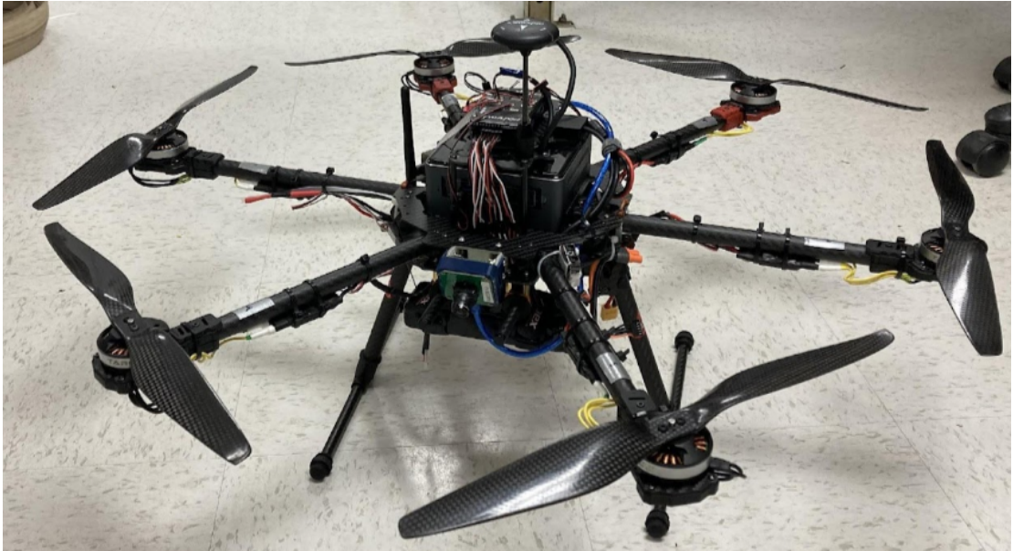
Figure 5.1: Fig. Physical hexacopter platform constructed to evaluate the effectiveness of the algorithm with. The system was fully developed, however experiments using the VaTF algorithm were not exercised.
