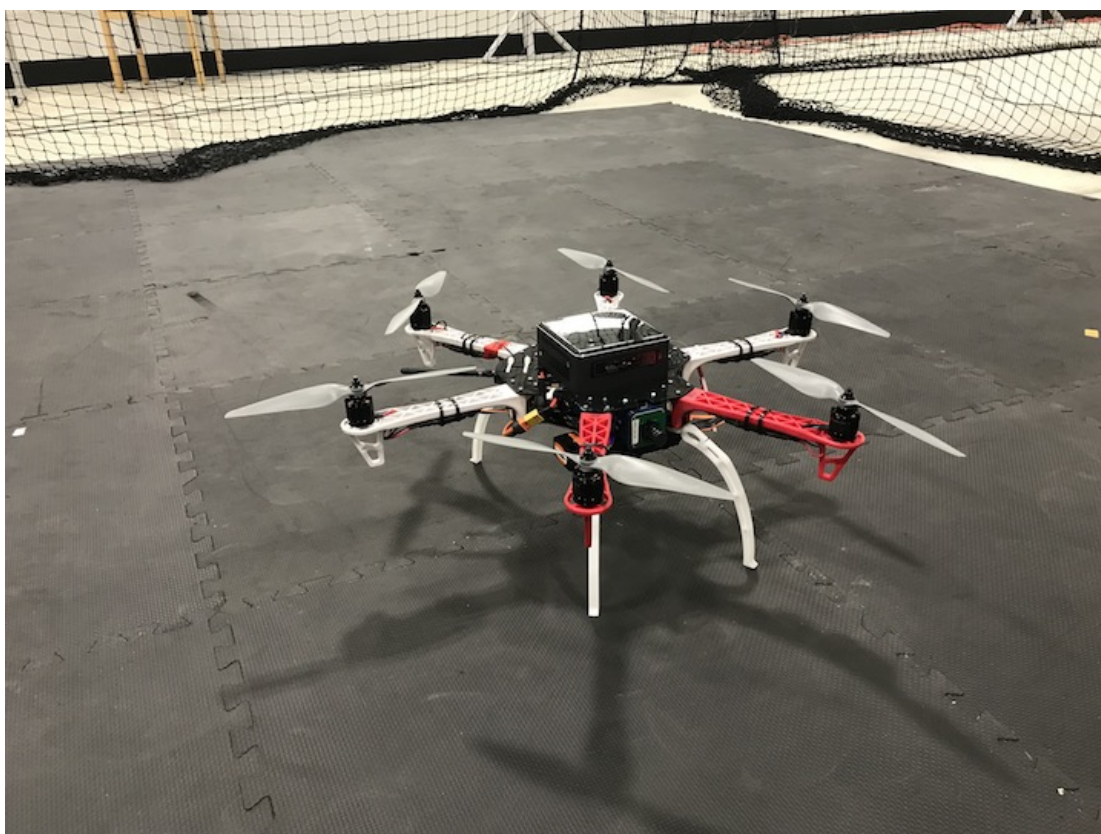
Figure 2.3: UAS used for ORB SLAM2 experiments. The payload includes an Intel NUC, mRo Pixhawk, Monocular Arducam, and various peripheral components.
