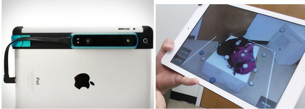
Figure 5.9: A 3D Structure sensor attached to a tablet (left) and the software interface of our simulation engine (right). The software can simulate the object dynamic with respect the gravity. The interface shows a scenario when we simulate balls fall onto an bag.
