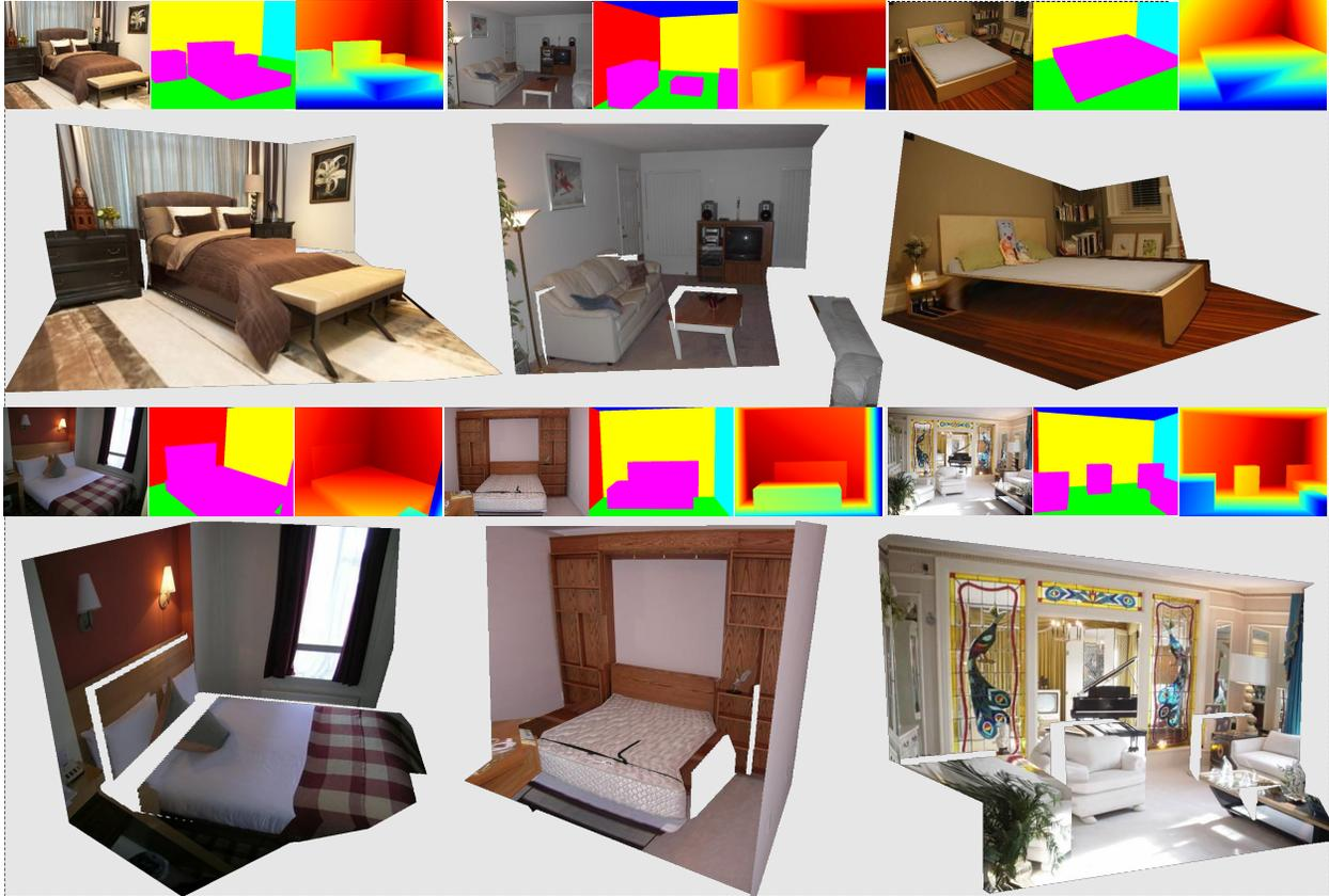
Figure 3.14: 3D reconstruction results based on 3d image parsing. For each image, we show an original image, a segmentation map, a recovered depth image, and a reconstruction result respectively.
