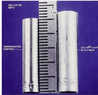
Figure 1.8: Unirradiated steel (left) and steel that has been irradiated for a year (right) [17].
