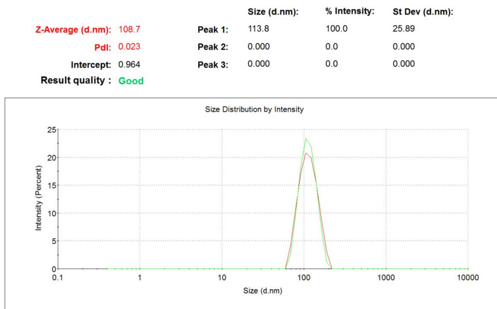
Figure 4.9: The average hydrodynamic diameter of 100-nm carboxylate-modified latex spherical beads measured by dynamic light scattering. The average hydrodynamic diameter is 114 +/- 26 nm.
