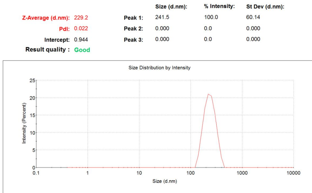
Figure 4.23: The average hydrodynamic diameter of elongated polystyrene templates with 2.3 aspect ratio measured by dynamic light scattering. The average hydrodynamic diameter is 242 \pm 60 nm.
