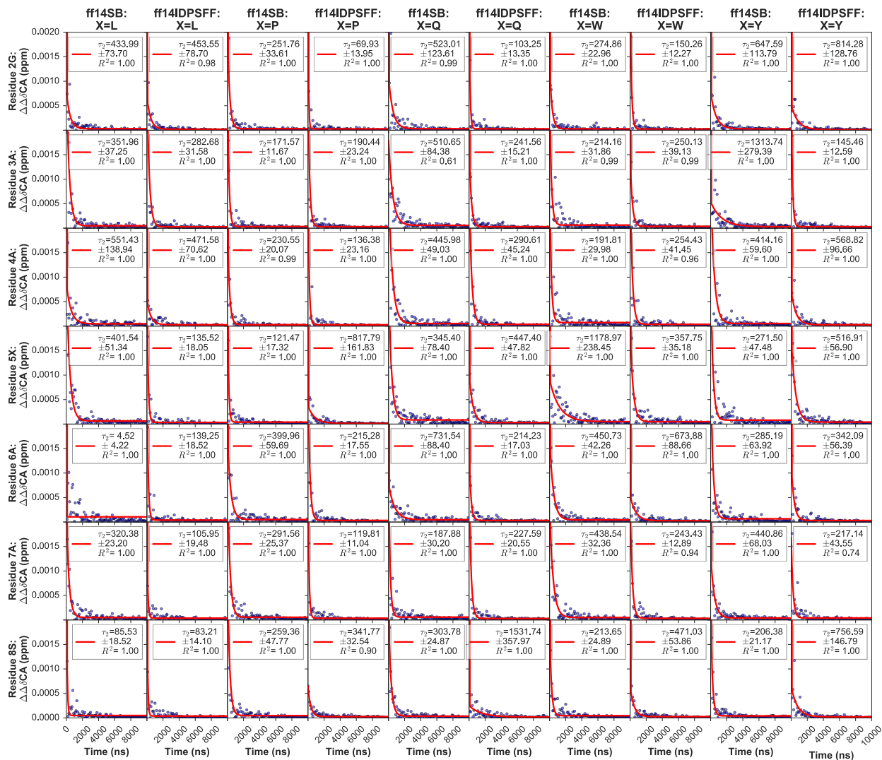
Figure D.7: Biphasic exponential fittings were generated using \Delta\Delta\delta C\alpha from cumulative average data in Figure D.1 for EGAXAASS (X= L, P, Q, W, Y) peptides and force field types. Each average cumulative \Delta\Delta\delta C\alpha (blue dots) 100-ns increment was plotted per residue. Datasets were fitted to the following exponential decay function: \Delta\Delta\delta C\alpha = A_1 e^{-\frac{t}{\tau_1}} + A_2 e^{-\frac{t}{\tau_2}} + c (red line). Each column represents a peptide and force field, and each row represents a single residue. Only residues 2G-8S are fitted.
