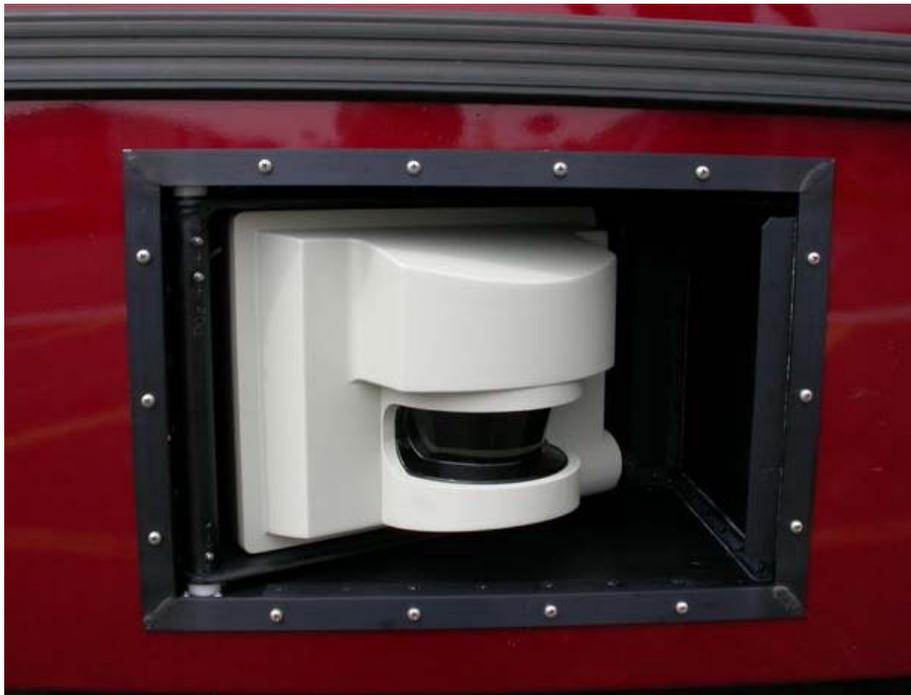
**Figure 12. SICK Laser Scanner and Retraction Assembly**
