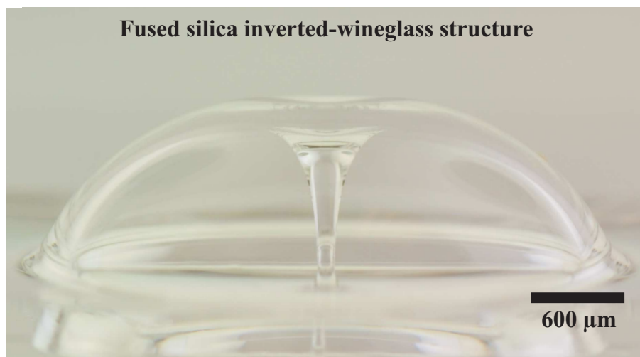
Figure 2.4: Optical photograph of glassblown fused silica inverted-wineglass structure. Outer diameter is 4200 μm. Glassblown at 1650 °C.
