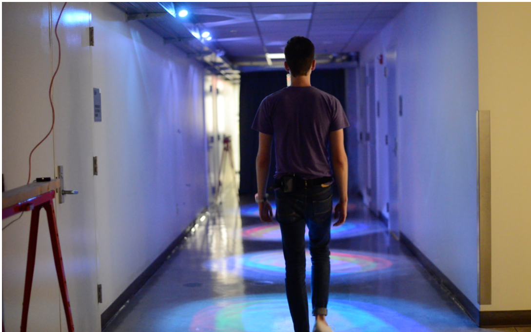
Figure 7.1: Experimental setup a) metrics: light radius = 1.12m, distance between lights = 2.7m, hallway width = 4m, hallway length = 30ft, base luminance with lights off = 2lx. Note: low illumination not displayed in this image; b) User walking with all lights on. Max luminance per light = 40 lx. Note: Image captured with high sensitivity camera, appears to be brighter than reality.
