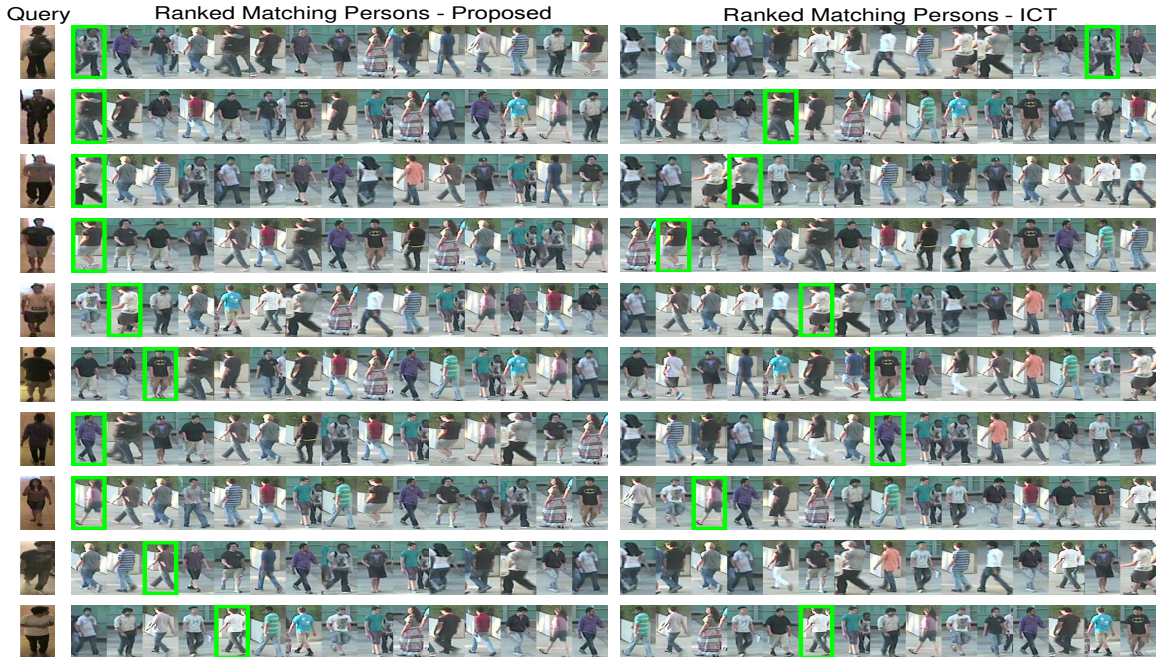
Figure 2.11: Visual comparison of matches using feature warps for camera pair 1-3 of the RAiD dataset. First column is the probe image. Second and third columns show the top 15 matches computed using the proposed method and ICT [5] respectively.
