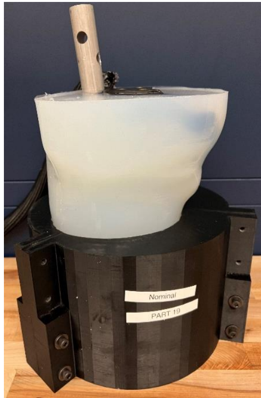
Figure 71: The demolding process, with the top sections removed first to avoid damaging the mold or silicone limbs.
