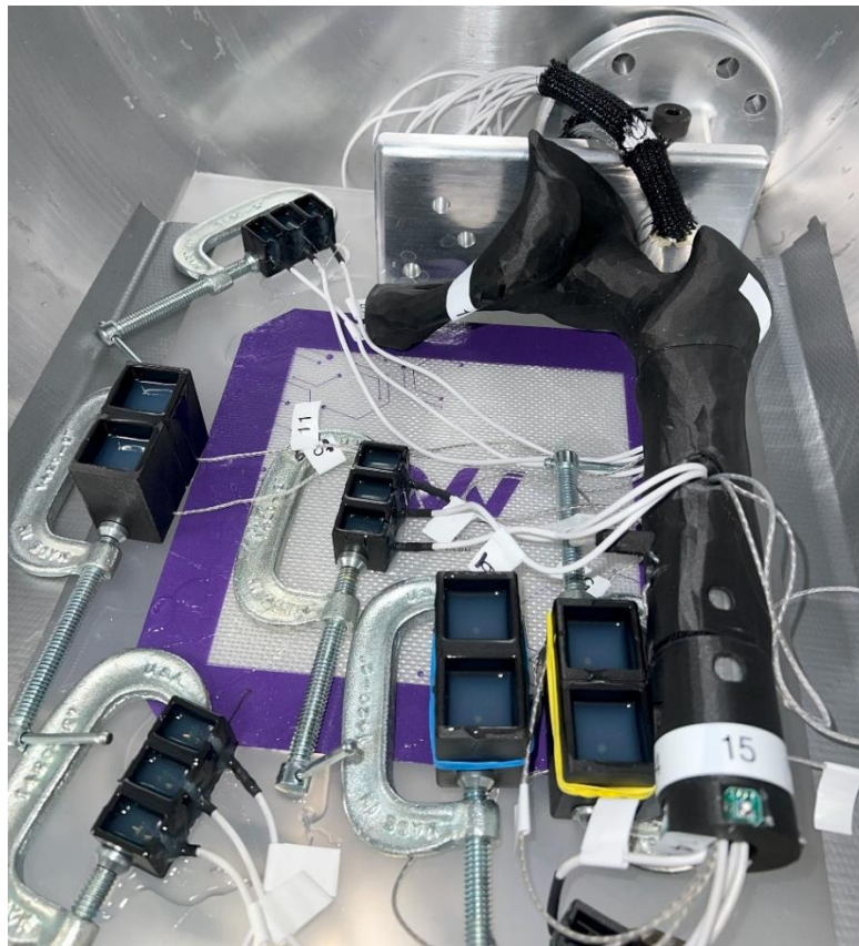
Figure 62: Pre-molded sonomicrometry and pressure sensors with the silicone poured into the molds.
