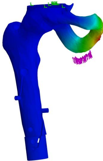
Figure 39: SolidWorks simulation deformation plots. The maximum displacement is experienced at the ischial tuberosity with a value of 2.923 mm.
