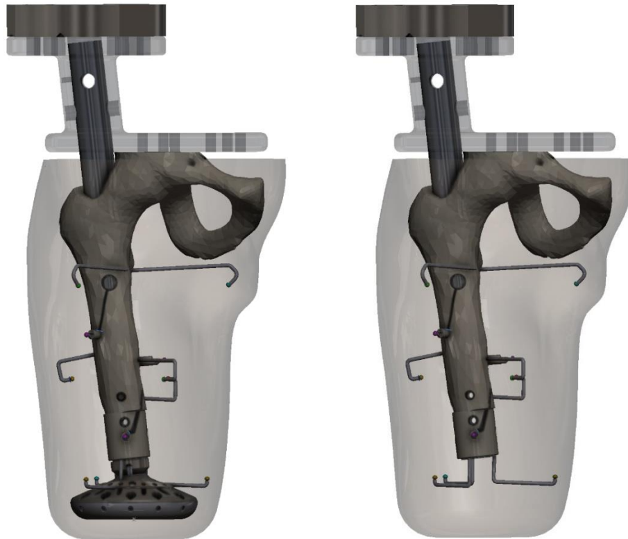
Figure 41: Final limb model with implemented sensors and wiring with(left) and without (right) the implant.
