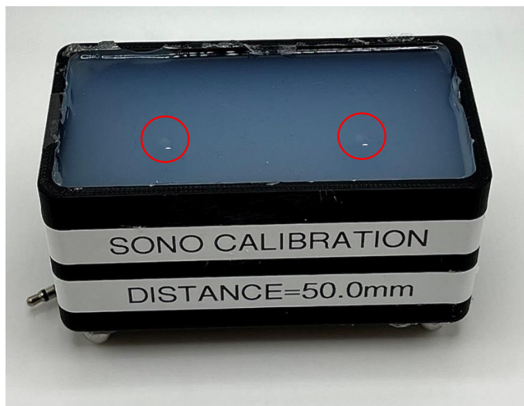
Figure 75: The apparatus used to calibrate the sonomicrometry device to the Ecoflex 00-31 silicone.
