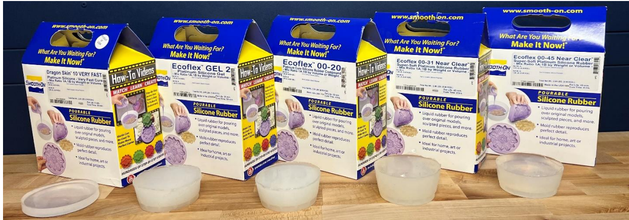
Figure 73: The various silicones tested for the limb from left to right: Dragon Skin 10, Ecoflex Gel 2, Ecoflex 00-20, Ecoflex 00-31 Near Clear, and Ecoflex 00-45 Near Clear.
