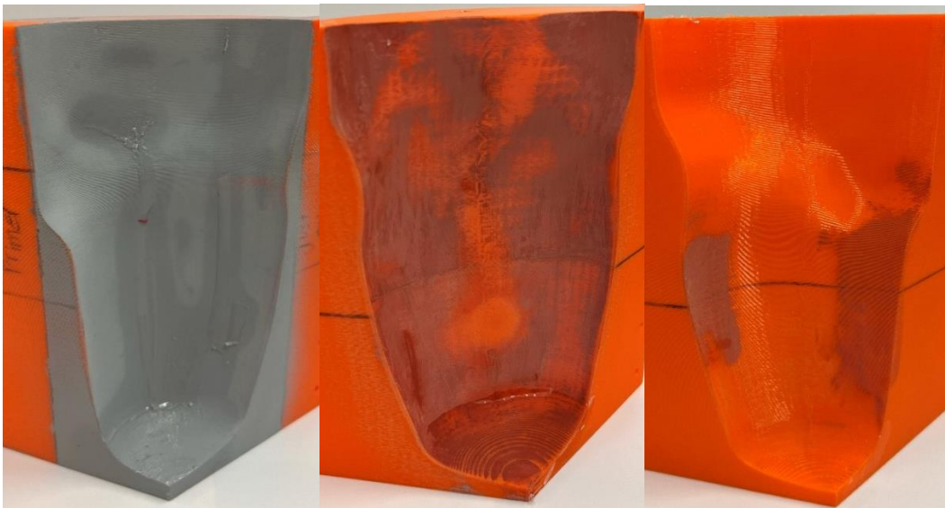
Figure 23: Various methods of improving the mold surface quality. 2 in 1 sandable primer (left), glazing spot putty (middle), sanding (Right).
