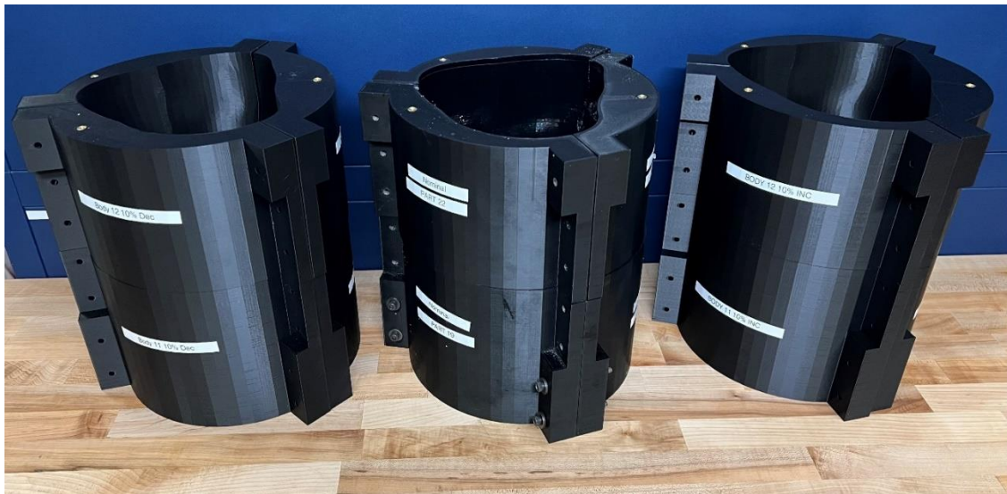
Figure 74: The 3D printed molds with three different inner volumes: -10%, nominal, +10%.
