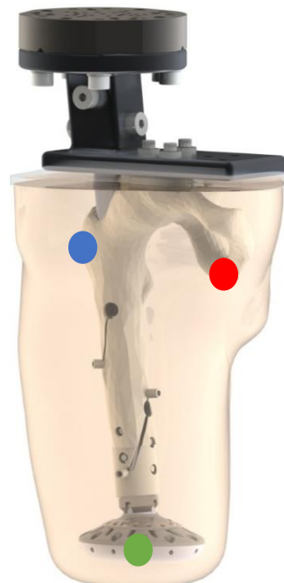
Figure 3: The Anatomical Engineering Group's sensorized silicone limb design. The ischial tuberosity and greater trochanter are marked with red and blue circles, respectively. The green circle represents the distal femur.
