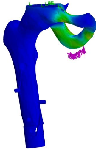
Figure 38: SolidWorks simulation stress plots. The maximum stress is experienced at the ischial tuberosity with a value of 1.796 \times 10^8 \text{ N/m}^2 . The maximum strain value was 8.047 \times 10^{-2} . This figure is exaggerated for visual purposes.
