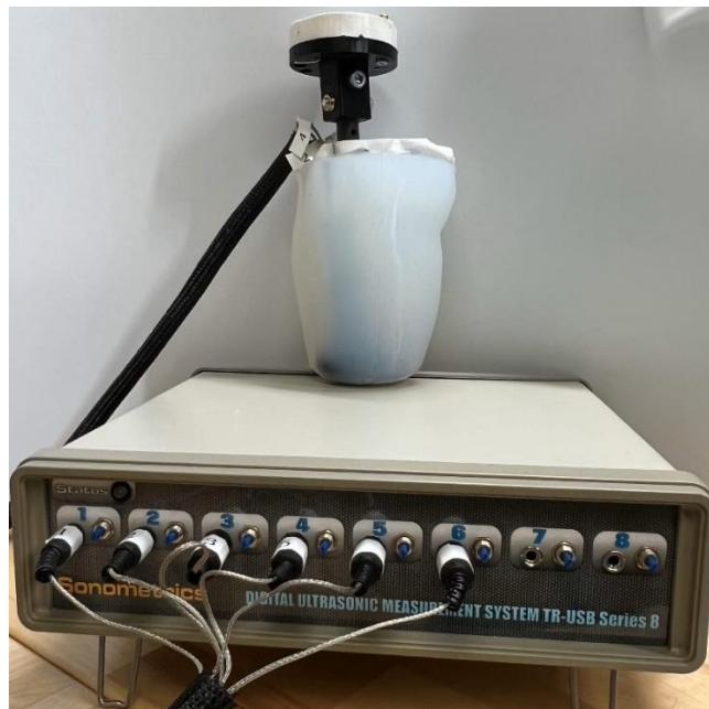
Figure 18: 8-Channel sonomicrometry device that was rented from Sonometrics.
