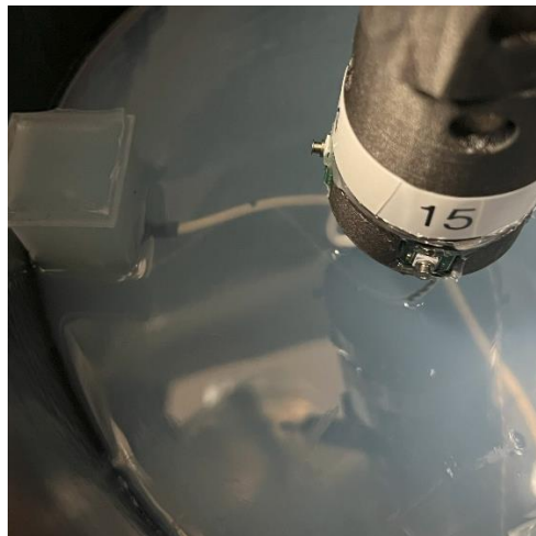
Figure 67: The first two levels of silicone with the bottom level of pressure sensors and sono crystals embedded.
