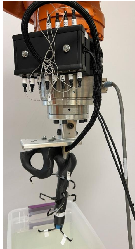
Figure 77: The sono water test experimental setup, including the breakout box and attachment, the KUKA attachment device, the model bone, and the aluminum tube and bone cover.
