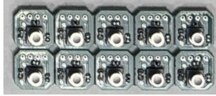
Figure 54: The 10 completed pressure sensors with two resistors, one capacitor, and one pressure sensor that were installed prior to being placed in the oven for the solder's melting.
