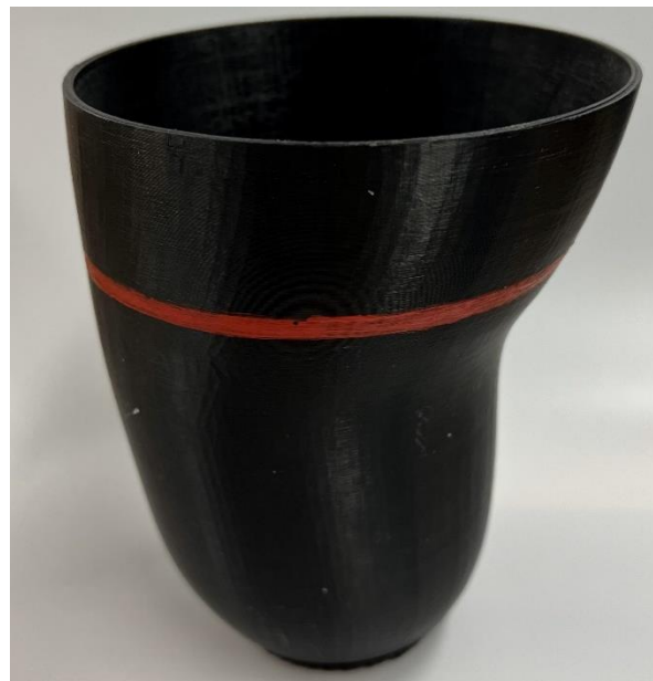
Figure 11: Preliminary single piece mold design utilized to construct the 1/2 scale limb.
