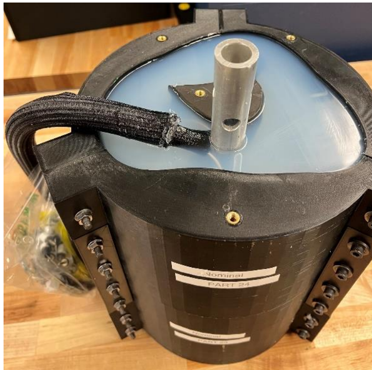
Figure 70: The final molding result with 7450 grams of cured silicone poured in ten sections.
