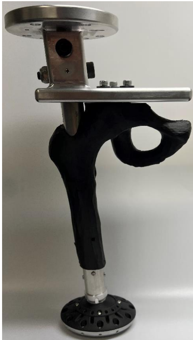
Figure 50: Model bone construction for the case with the ferromagnetic implant.
