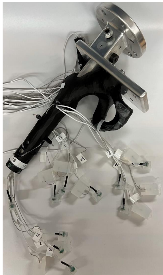
Figure 63: The sensors encased in silicone prior to the final molding processes.
