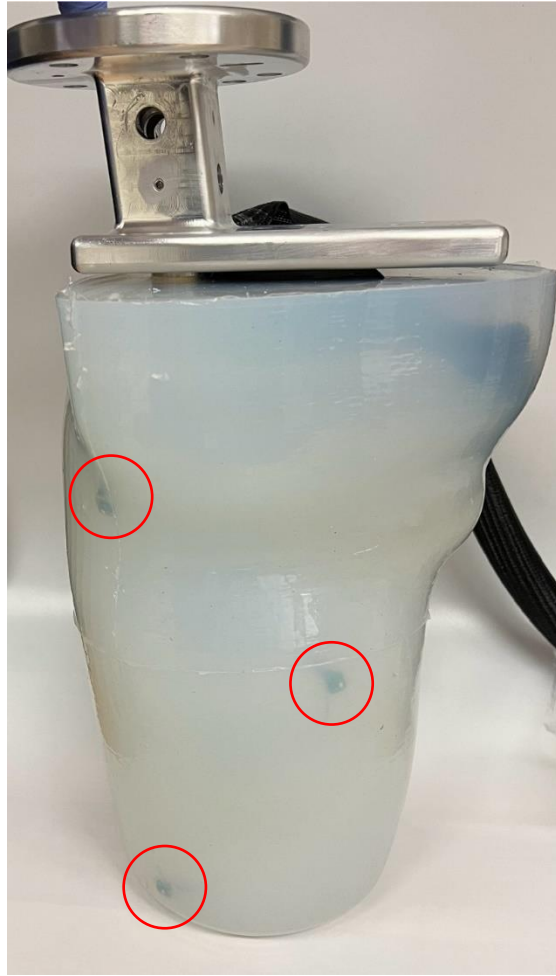
Figure 72: The final sensorized model limb with the KUKA attachment mounted. The red circles highlight the implanted pressure and sono crystals on this side of the limb.
