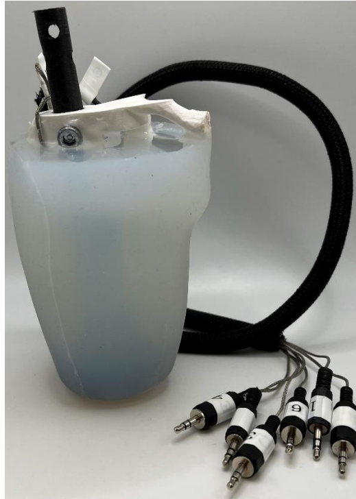
Figure 20: Secondary half-scale design with implanted sonomicrometry sensors.
