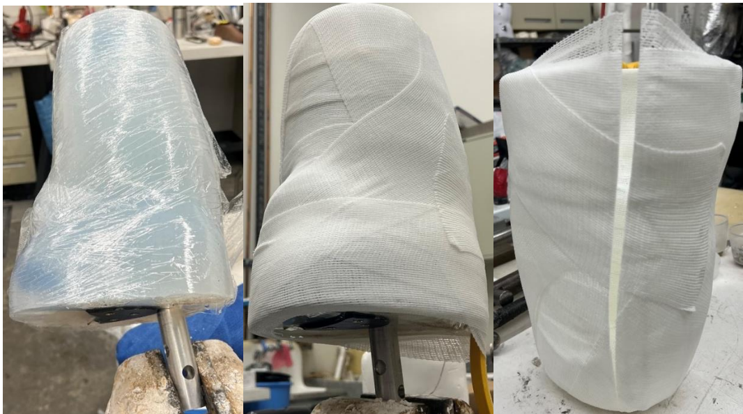
Figure 92: The initial stages of making a check socket for the sensorized silicone limb model detailed in this report. The UCLA Prosthetics and Orthotics Center has created a limb positive of our model limb in preparation to build the check socket.
