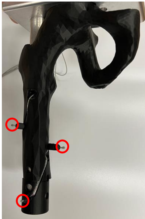
Figure 60: The sono ground crystals 1, 2, and 3 (highlighted by the red circles) were the first to be installed; these crystals were tested in water to confirm their functionality.
