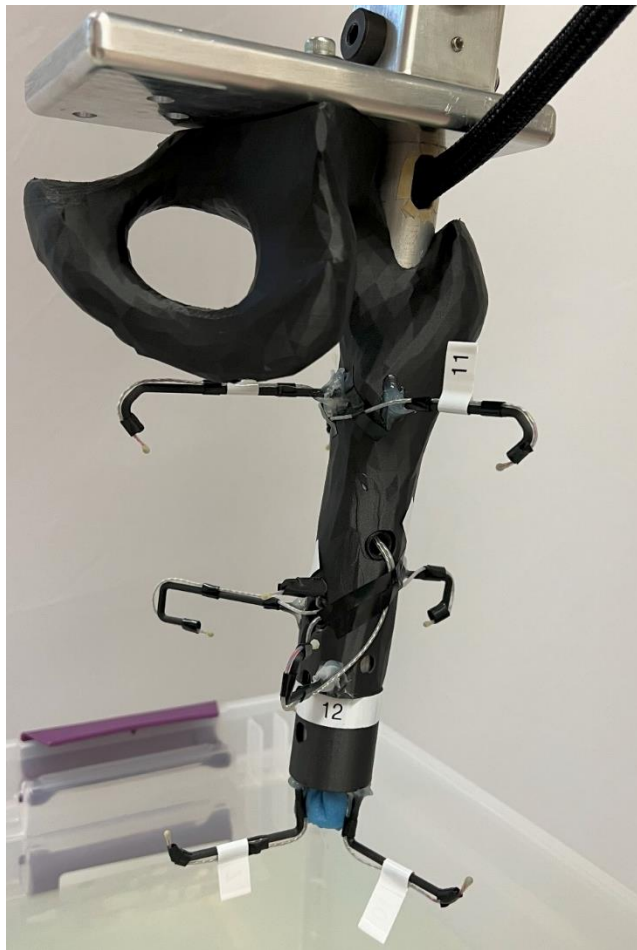
Figure 76: The sono water test model used to validate the crystal placement. Three crystals are grounded, and nine crystals are attached to their respective connectors, representing the wire length.
