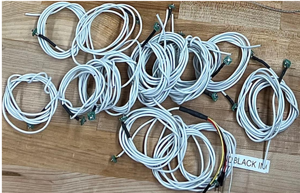
Figure 56: The 16 finalized pressure sensors with the shielded wiring installed.
