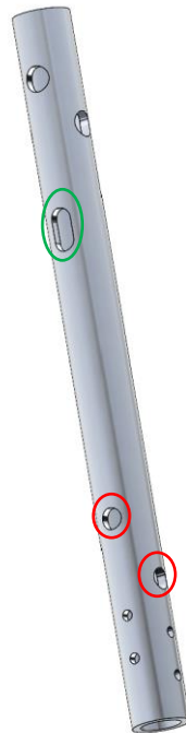
Figure 32: Aluminum tube design with various hole sizes and locations. The sensor wires will enter the tube from the slot location (green) and exit throughout the limb at the designated locations (red).
