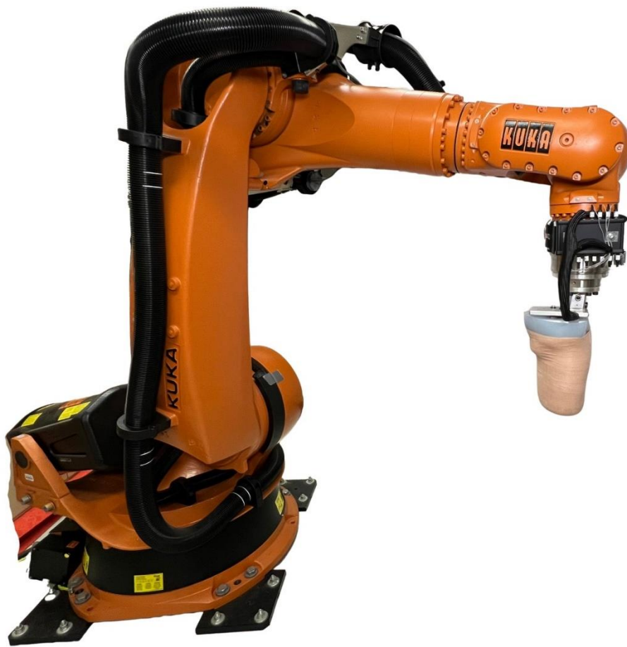
Figure 82: The final image with the sensorized model limb attached to the six-axis KUKA robotic arm.
