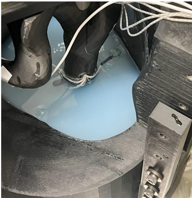
Figure 69: Mid-level sensors with silicone poured to the top of level 5 in preparation for level 6.
