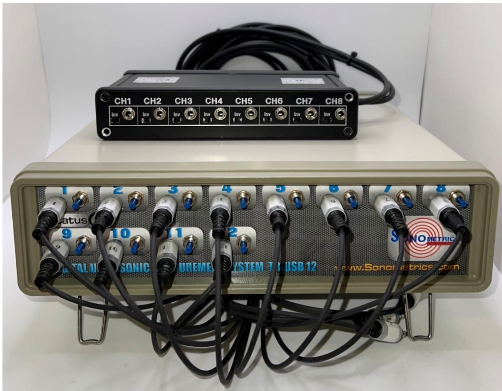
Figure 42: Digital 12-channel transceiver sonomicrometer hardware from SonoMetrics Corporation. An additional 12-channel breakout box is used to extend the sensors wire lengths. The device costs $16,000, and the breakout box costs $700.
