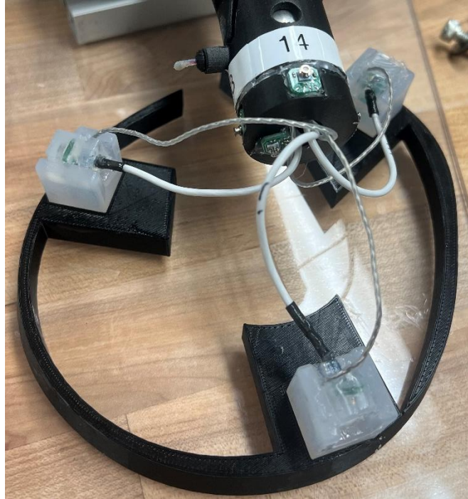
Figure 66: The stencil used to position crystals 7, 8, and 10 with their respective pressure sensors on the bottom level of the limb.
