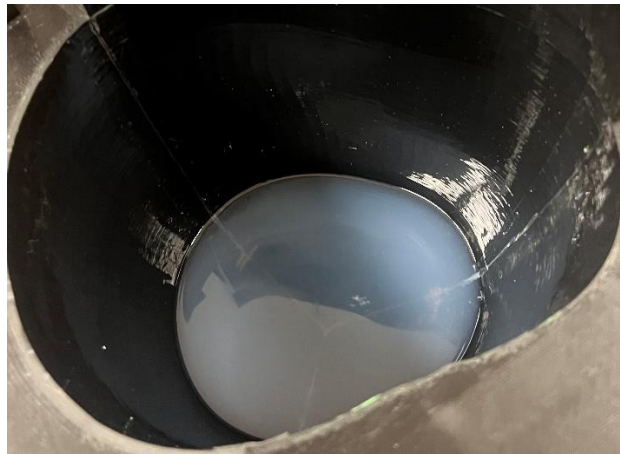
Figure 65: The initial 200-gram silicone pour preventing wires from sticking through the bottom of the limb.
