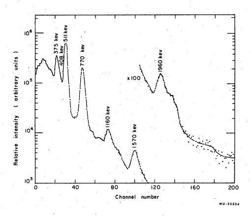
Fig. 2. Gamma-ray spectrum of 34-h Sr<sup>83</sup> taken with a 7.6-cm x 7.6-cm NaI(Tl) crystal. A 0.75-cm carbon absorber was placed between the source and crystal to reduce bremmstrahlung and annihilation-inflight photons caused by the positrons.
