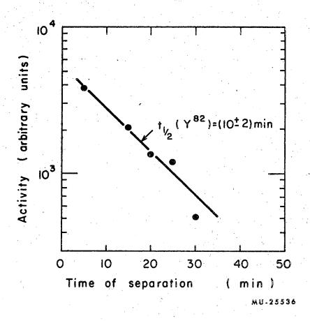
Fig. 1. Yields of 2.0- to 3.0-Mev positrons of Sr 82-Rb decay as a function of time of chemical separation of strontium from yttrium parent.
