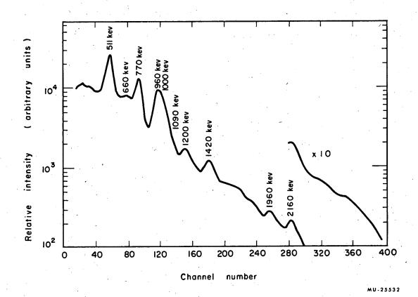
Fig. 4. Collimated photon singles spectrum of 39-min Y84 taken with a 7.6-cm x 7.6-cm NaI(T1) crystal.
