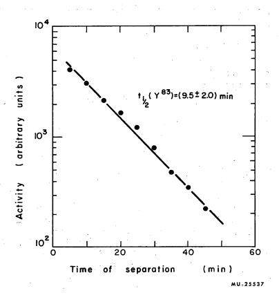
Fig. 3. Yields of the 375-kev gamma ray of  $\mathrm{Sr}^{83}$  as a function of time of chemical separation of strontium from the parent yttrium.
