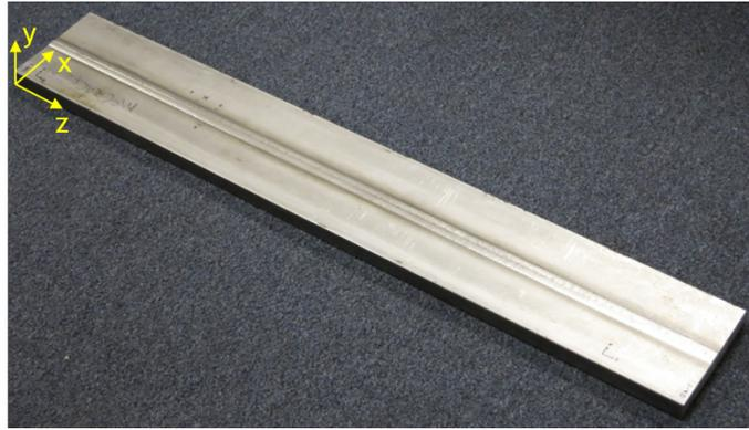
*Fig. 1 – Photo of the full stainless steel dissimilar metal welded plate that the slices were removed from. The plate has global dimensions of approximately 1220 mm x 152 mm x 25.4 mm (48 in x 6 in x 1 in) (excluding weld bead). Slices were removed near the mid-length of the plate and have a thickness of 6.35 mm (0.25 in)*
