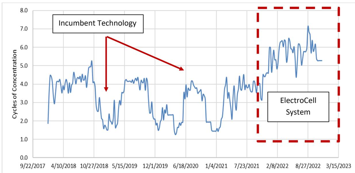
Figure 14. Cycles of concentration, incumbent versus ElectroCell systems
