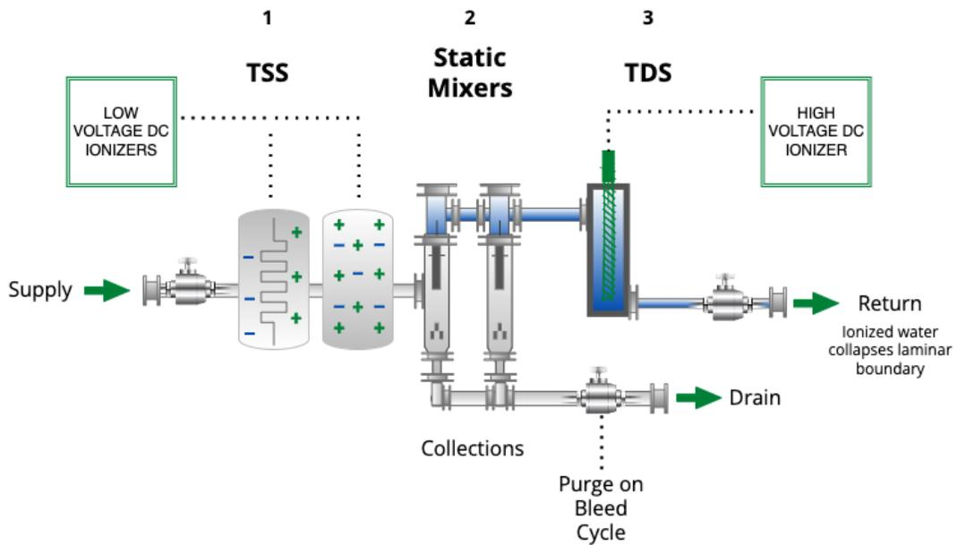
Figure 3. The three-stage ElectroCell system
