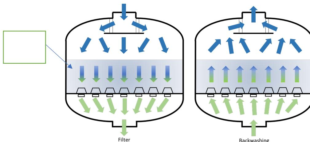
Figure 1. Pressure sand filter technology
