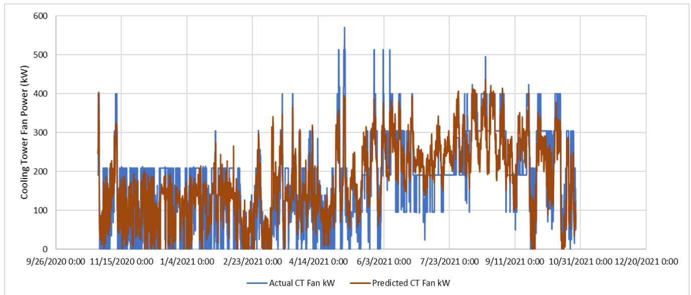
Figure 9. Actual versus predicted cooling tower energy use for the incumbent system
