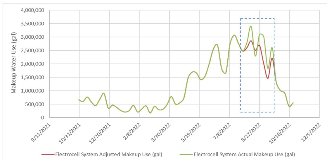
Figure 13. ElectroCell system adjusted makeup water use
