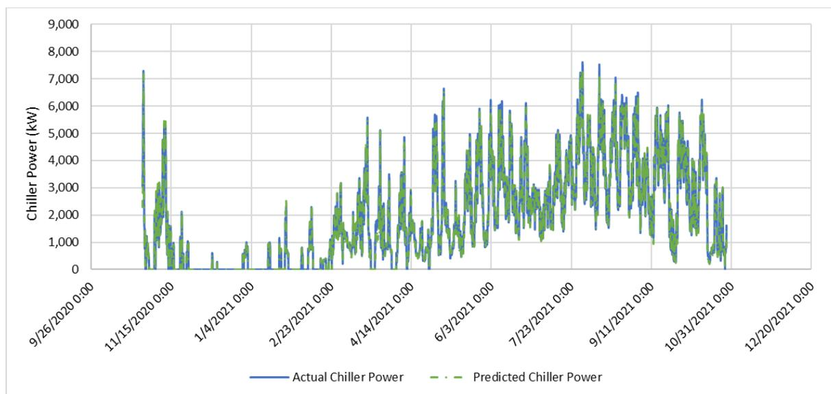
Figure 8. Actual versus predicted CHW energy use for the incumbent system
