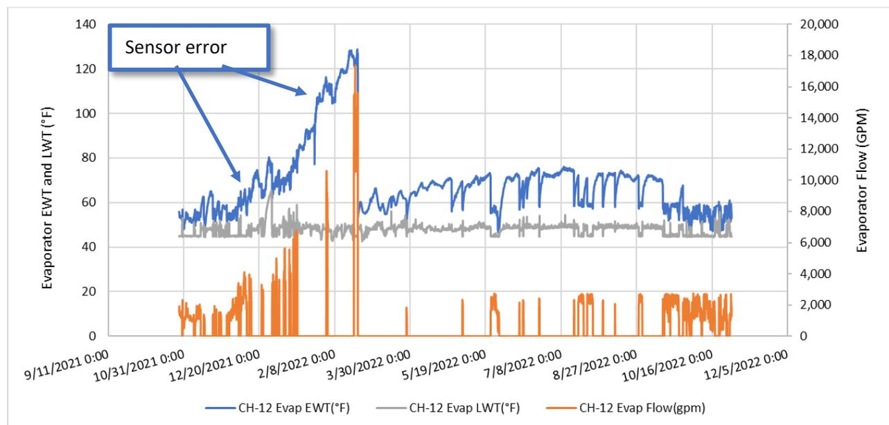
Figure 6. Chiller 12 temperature data from ElectroCell performance period
