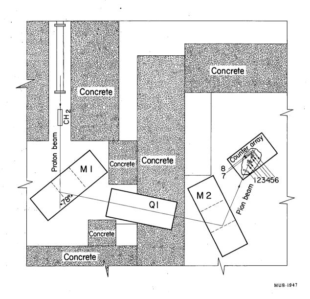
Fig. 1. Pion-beam magnet system and counter array.
