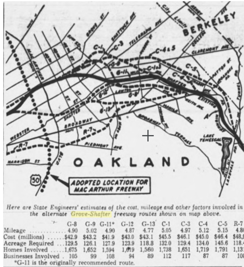
Figure 2.6. 144 Map of the proposed Grove-Shafter routes with calculations on homes and businesses that would be moved or razed given each selection.
