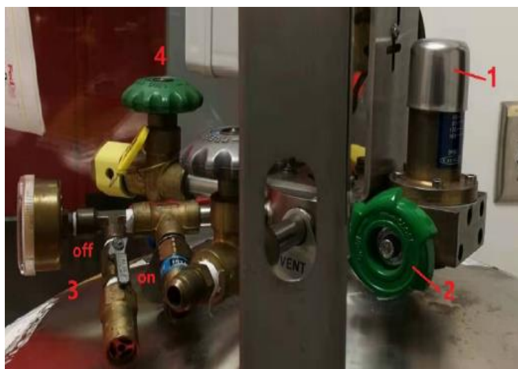
Figure A4.1 FTIR N 2 purge gas and liquid N 2 tank configuration (adapted from Z. Loh, 2010).
