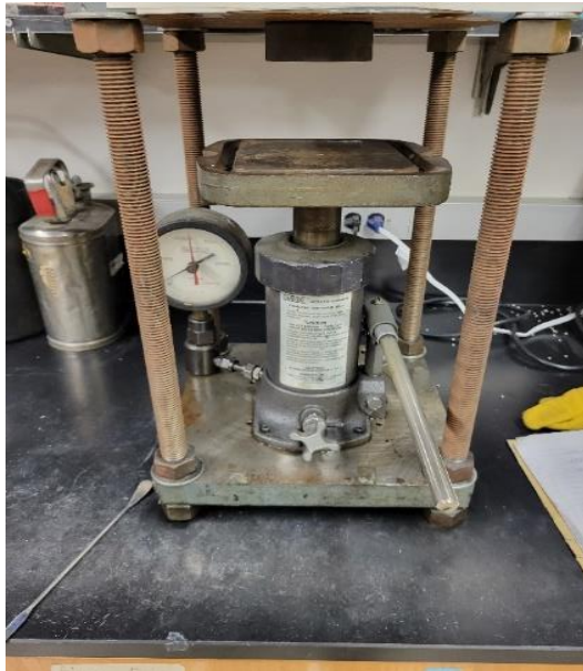
Figure A3.1 Hydraulic press in YH 1043 with maximum pressure limit of 10,000 lb
