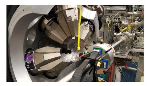
Figure 2.12: The Gamma-Ray In-beam Nuclear Array, GRETINA
