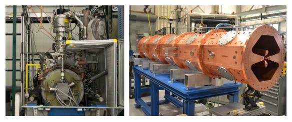
Figure 2.2: The Electron Cyclotron Resonance ion source (left) and Radio Frequency Quadrapole (right). [26]
