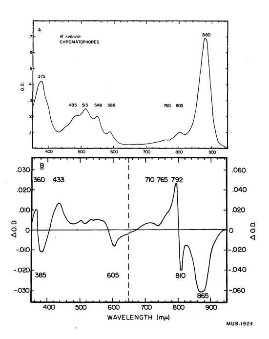
Fig. 3A. Absorption spectrum of R. rubrum chromatophores suspended in 0.01 M phosphate buffer, pH 7.13; 1 cm cuvette.
