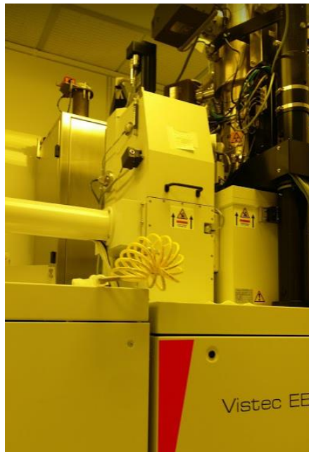
Figure 3-2: (a) Electron beam lithography and (b) Focused ion beam and scanning electron microscopy systems used for fabrication of the samples.
