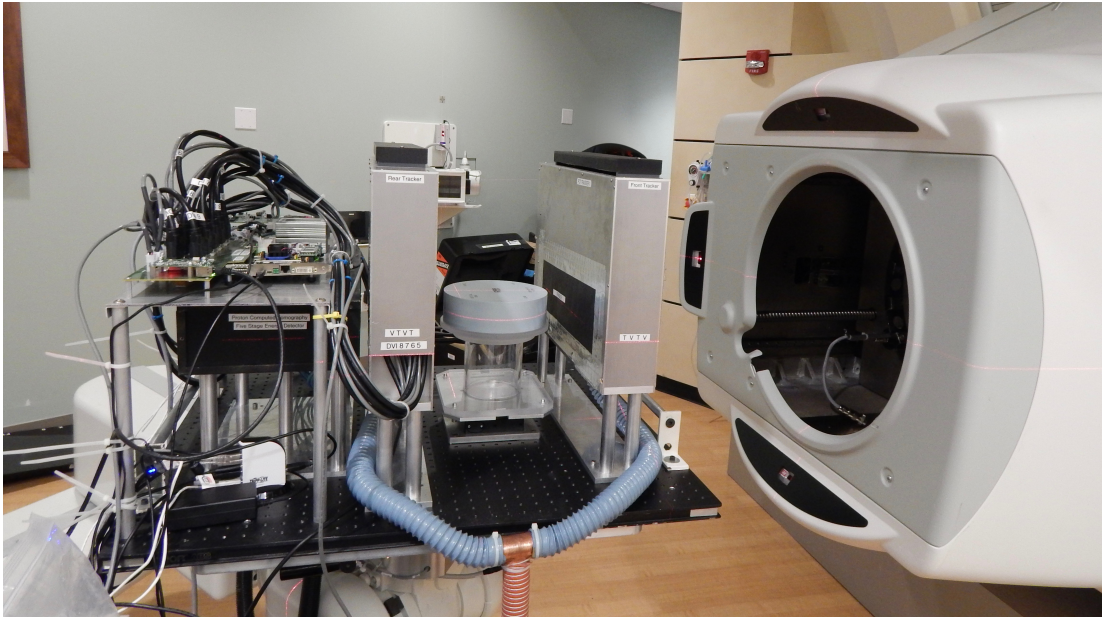
Figure 7.4: Prototype proton CT scanner installed on the fixed horizontal beam-line at NMCPC with the edge phantom mounted on the rotation platform.
