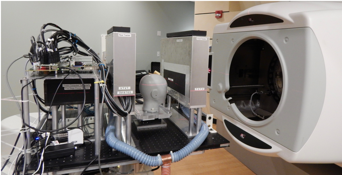
Figure 6.3: The anatomical pediatric head phantom installed on the beamline at NMCPC.
