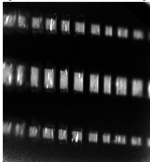
Fig. 2 X-ray microscope image in reflection mode of a test sample taken at 7.5 degree incidence angle. The dark regions have been milled by FIB to reduce the reflectivity. The image covers an area of approximately 10 microns vertically and 100 microns horizontally.
