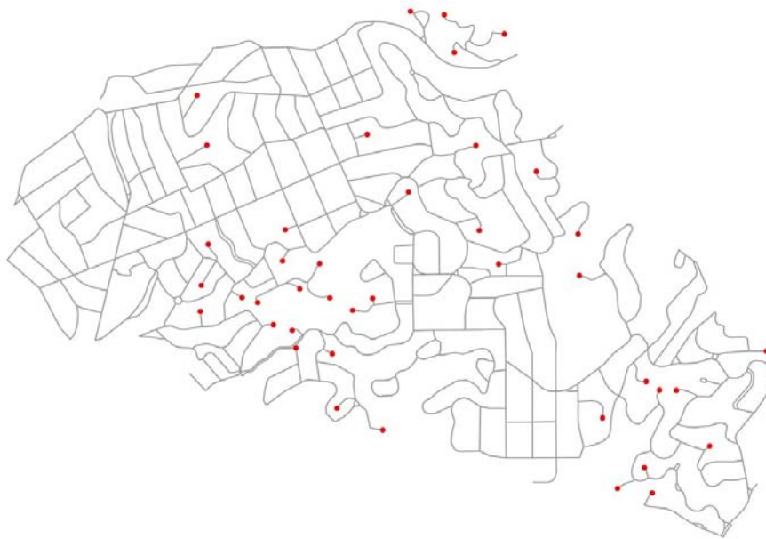
Figure 5.8. OSMnx visualizes the spatial distribution of dead-ends in the city of Piedmont, California.
