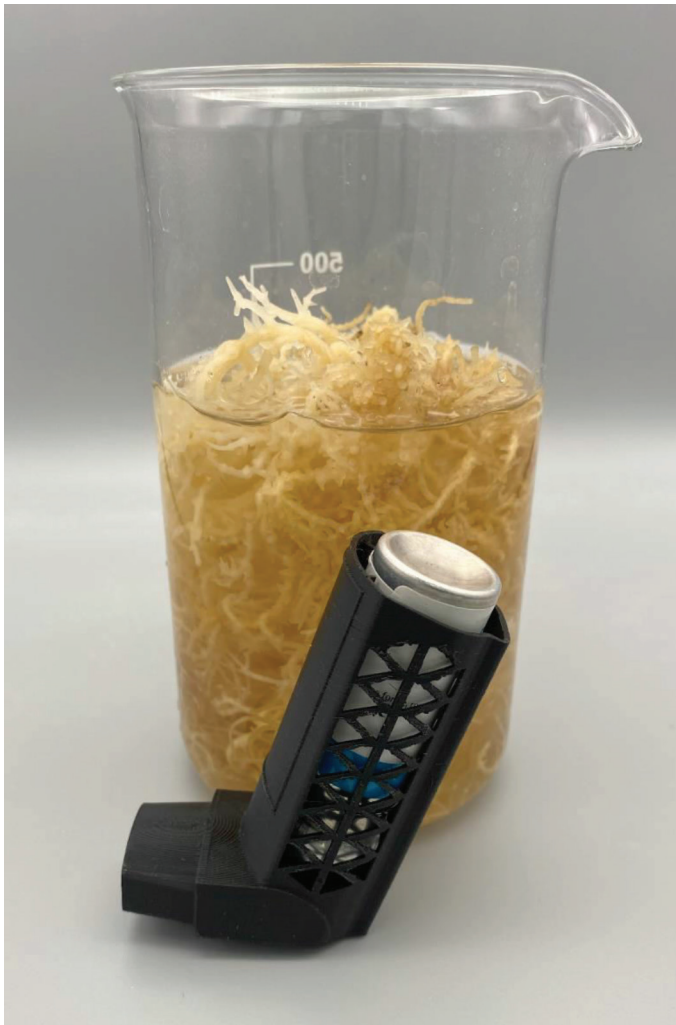
Figure 3 Seaweed-based biomaterial used to 3D print inhaler prototype (front), set against a jar of the seaweed, used as an alternative feedstock to fossil fuels used in current medical device manufacturing (back). Source: with permission: Symbio-tex ( https://www.symbio-tex.com/ ).
