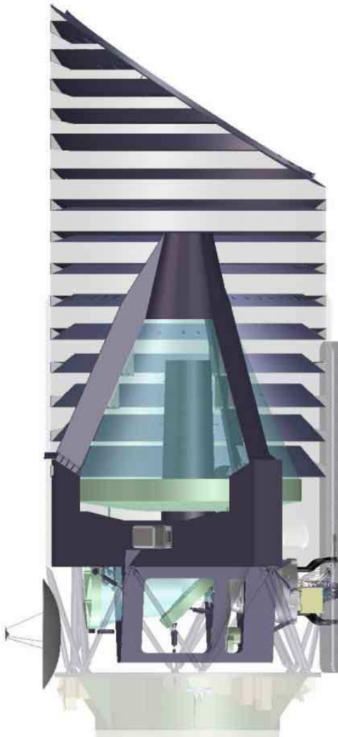
Fig. 14.— Schematic treatment of the outer baffle interior vane arrangement. Sunlight is incident from the left, where the height of the baffle and its angled forward edge maintains the baffle interior in darkness.
