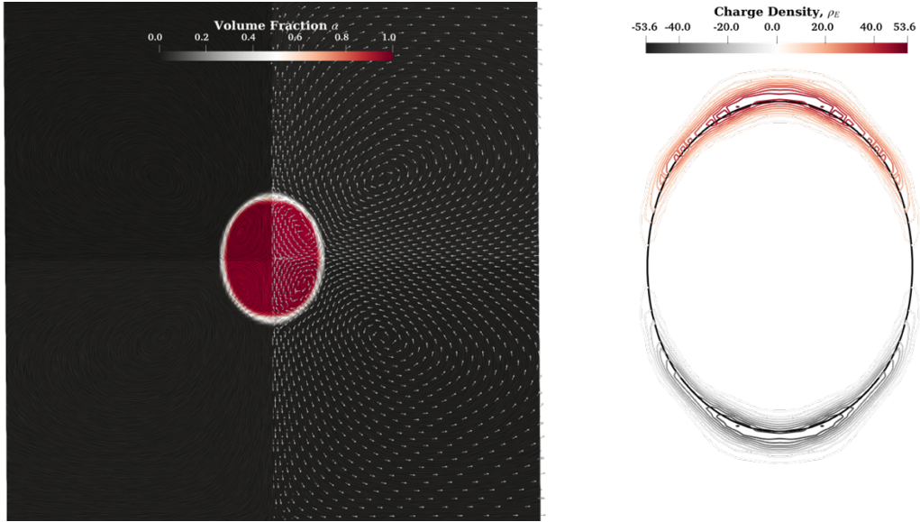
Fig. 21 Prolate deformation of droplet at Ca_E = 0.625 . Left: Streamlines are shown using a Surface Line Integral Convolution (LIC) representation. Right: Iso-contours of charge density around droplet interface.
