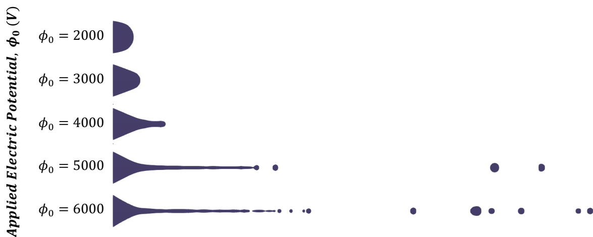
Fig. 33 Cone-jet profiles for various values of \phi_0 at t = 6 \text{ s} and f = 1 .
