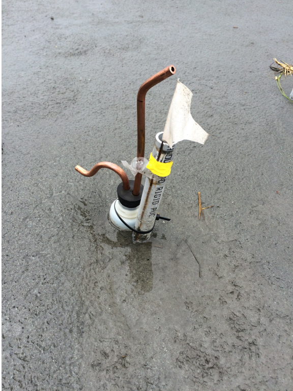
Figure 2: Single Stage Sampler Bottle zip tied to PVC pipe on experimental site.
