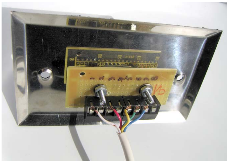
Figure 9.5. HVAC Interface, rear of wall-mount
