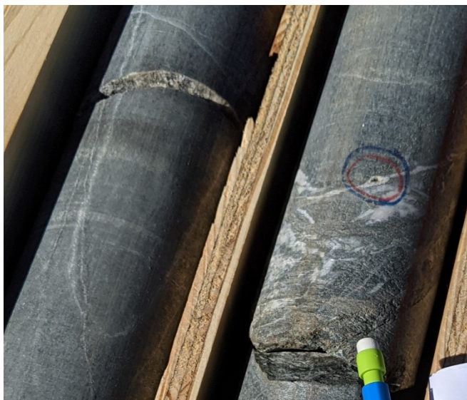
Figure 7. Single vuggy pore, ~207' (63.1 m) depth, E2-TS. An attempted permeability measurement using a NER "Tinyperm" permeameter was unsuccessful because values were below the instrument's limit.
