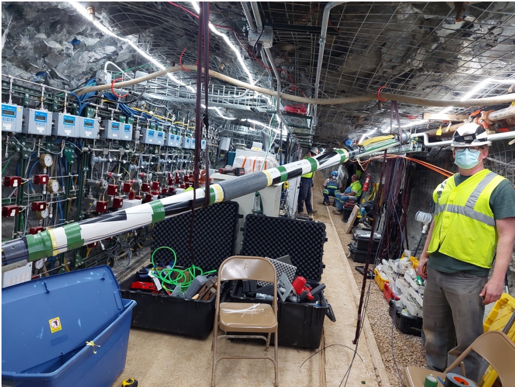
Figure 5.2. ERT/DORSA tools. Top: ERT electrode on PVC Shroud. Bottom: DORSA added to ERT shroud.
