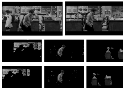
Fig. 3. Notting Hill sequence. (Row 1) Original image pair of size 311 \times 552 , (Row 2) Pixels assigned to warp layers 1-3 in I , (Row 3) Pixels assigned to warp layers 1-3 in I' .
