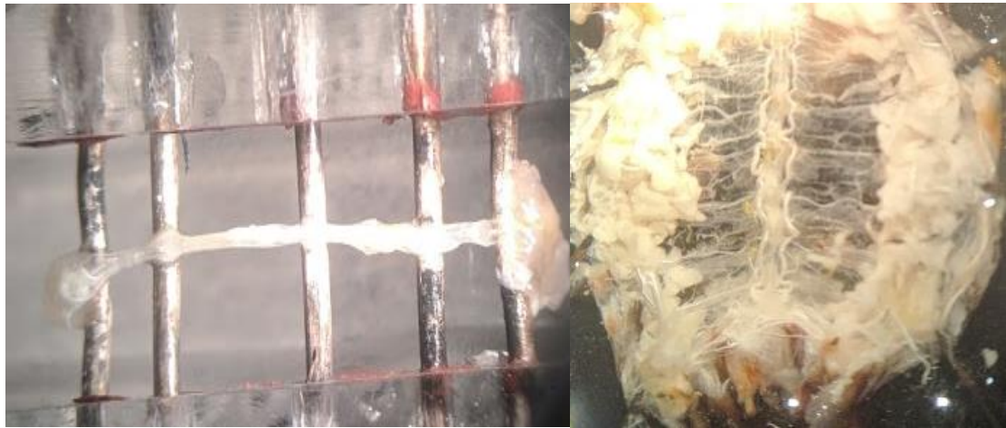
Figure 4.1 Cockroach nerve cord. a) Cockroach nerve cord over electrodes. The left two electrodes are the stimulation. The right two are the recording electrodes and the middle electrode is the ground. b) The dissection of the cockroach showing the nerve cord.
