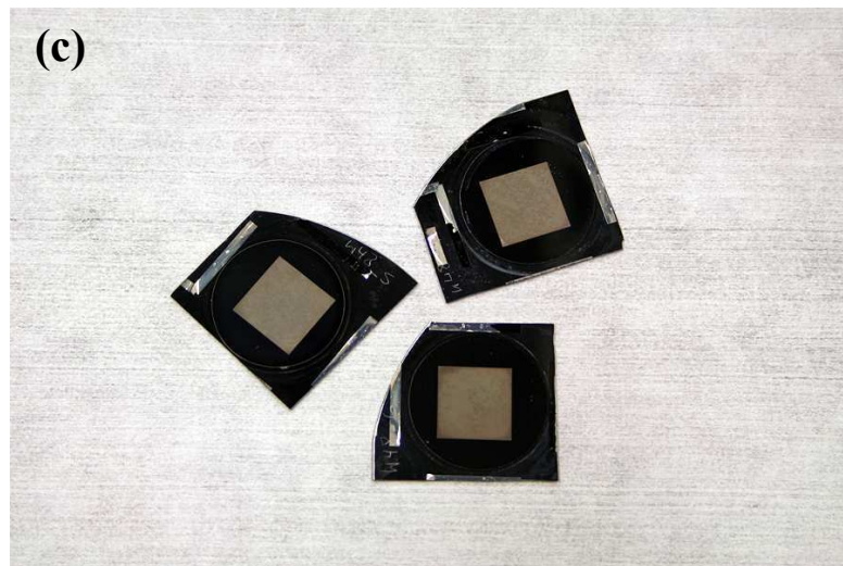
Figure 4.5 (a) Samples being loaded into the plasma etch rig. (b) A sample seen through the viewport during the etch process. The viewport allows for real-time monitoring of the process. (c) Samples after the plasma etch (Fig. 3.1 e). Images by L. Gu.
