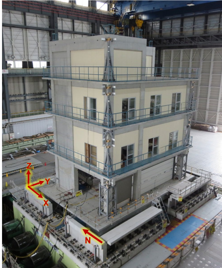
Figure 5.1. Base-isolated building specimen with moat walls.
