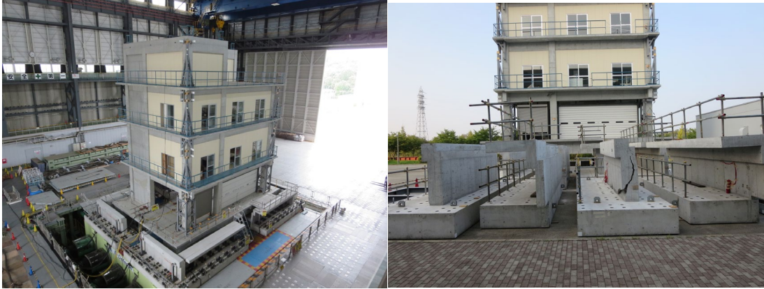
Figure 2.22. Left : Overview of base-isolated building specimen. Right : Moat walls damaged from pounding events. Photo credit: Hirohisa Fukui, E-Defense.
