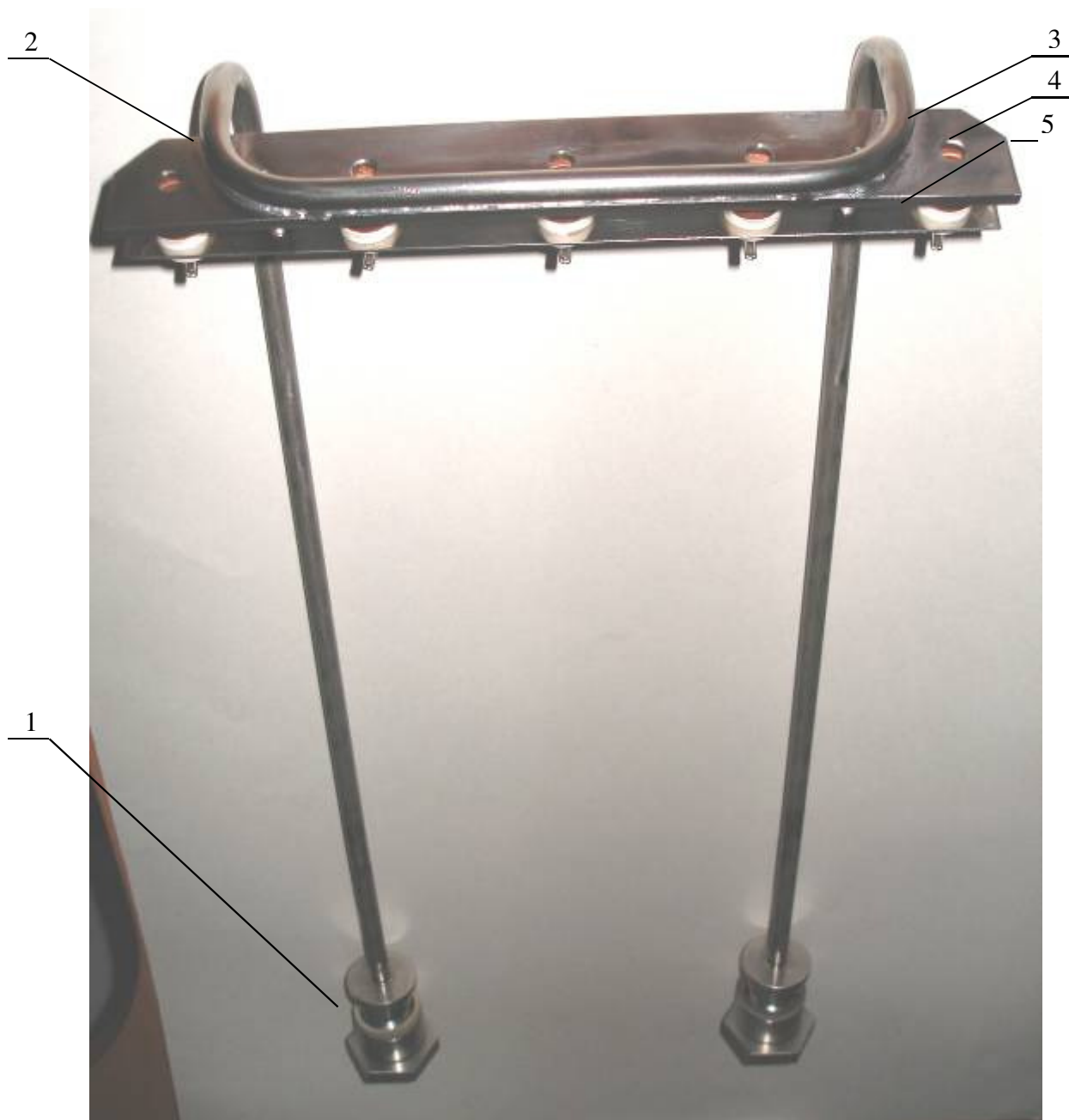
1 – input fitting; 2 – water pipe; 3 – screen; 4 – диафрагма; 5 – Faraday cup
