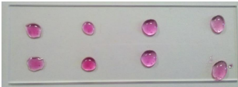
Figure 71. Example slide (Teflon-coated) showing eight droplets: four contain media with Pluronic, and four contain media without Pluronic.
