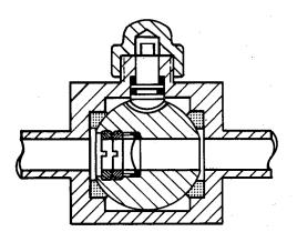
Fig. 3. Rupture-disk ball valve.
