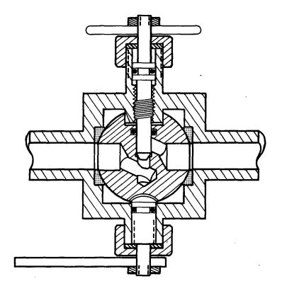
Fig. 6. Needle ball valve.
