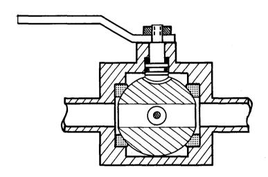
Fig. 2. Fail-safe ball valve.
