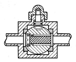
Fig. 4. Strainer or filter or dryer ball valve (strainer is shown).
