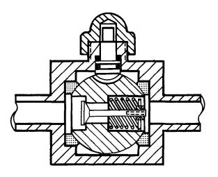
Fig. 5. Relief (or check) ball valve.
