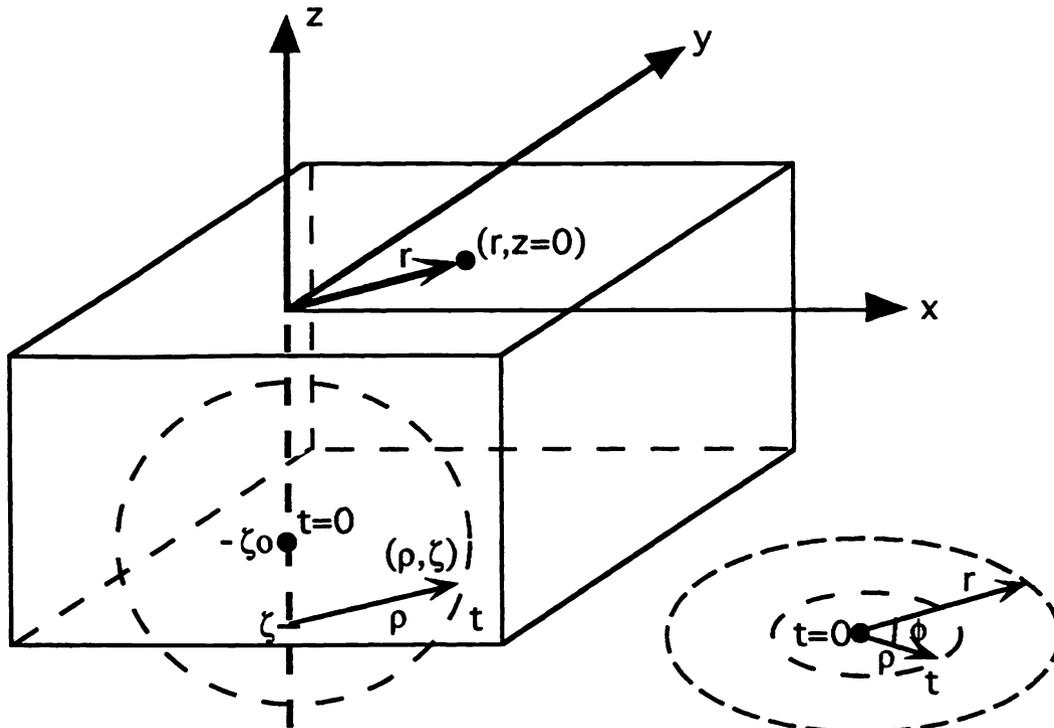
Figure 2: Geometry assumed for PTT point spread function computation.
