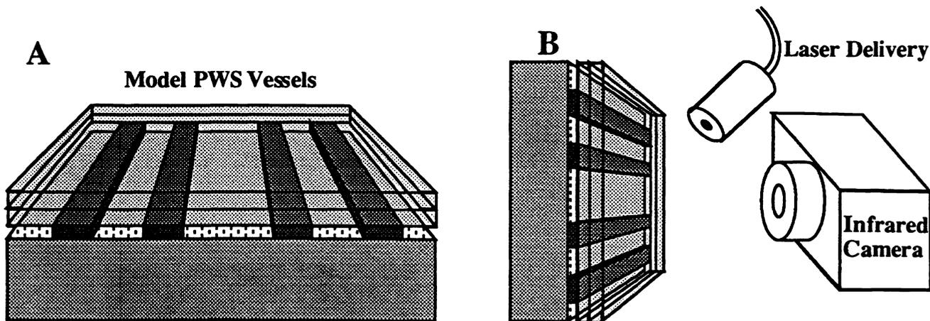
**Figure 3:** (A) Model collagen phantom simulating buried PWS blood vessels. (B) Experimental arrangement to test resolution of PTT.
