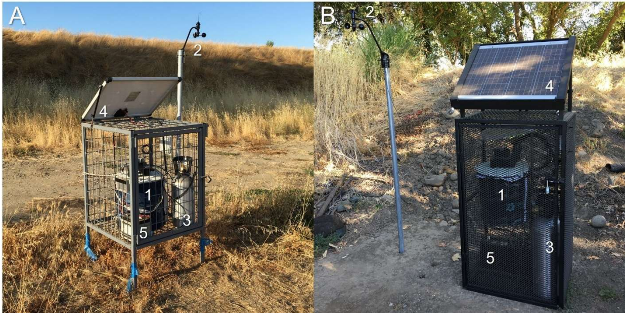
Figure 2.2. Examples of the BG-Counter trap configurations. Panel A shows the cage design in Sacramento-Yolo MVCD while Panel B shows the design in Placer MVCD. All traps were fitted with 1) a BGC trap, including the infrared sensor and temperature recording device.; 2) an anemometer and wind vane recording wind speed and direction every 1 minute; 3) a 20-lb CO 2 cylinder; 4) a solar panel; and 5) a 12V battery for powering the trap.
