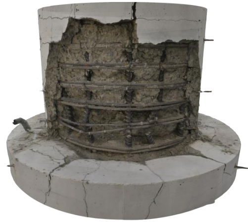
Figure 2–29: Damage after the completion of the test at the north face (Lotfizadeh, 2019).
