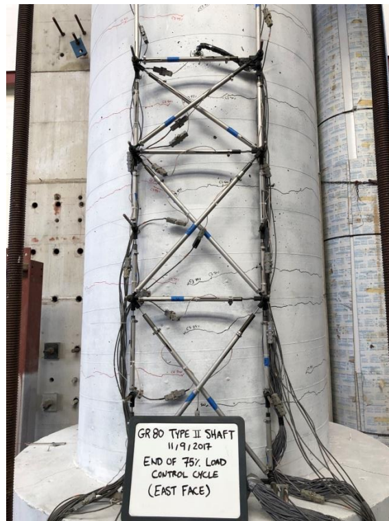
Figure 2–28: Picture of test-specimen at the shaft column interface at the end of the 75% load control cycle (Lotfizadeh, 2019).
