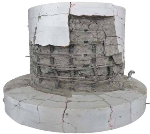
Figure 2–29: Damage after the completion of the test at the north face (Lotfizadeh, 2019).
