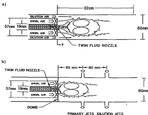
FIG. 1. Model combustors
