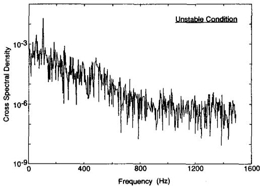
FIG. 4. Cross-correlation of the acoustic and radiometer signals for an unstable condition
