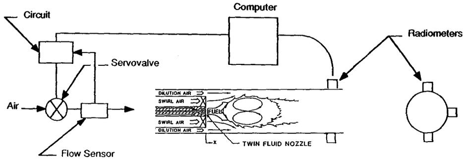
FIG. 2. Overall approach to active reduction of soot loading in the ASCC
