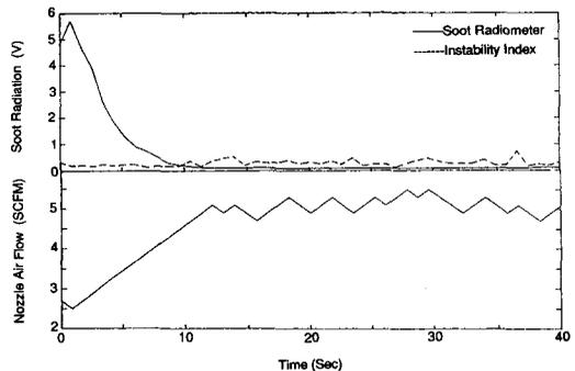
FIG. 5. Soot radiometer, stability index, and nozzle air flow vs. time
