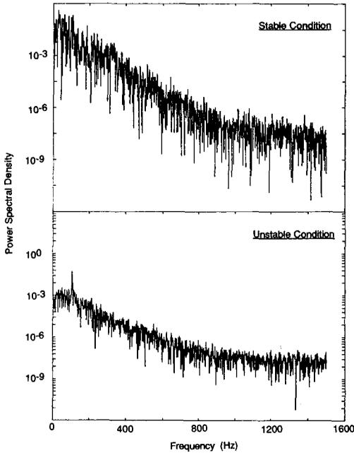
FIG. 3. Power spectral densities of radiometer and acoustic data for stable and unstable conditions
