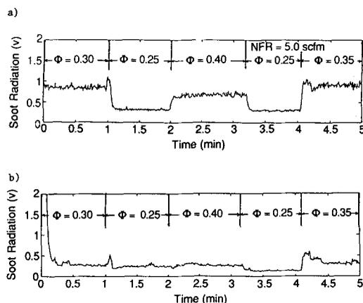
FIG. 6. Non-optimized and optimized performance in the ASCC
