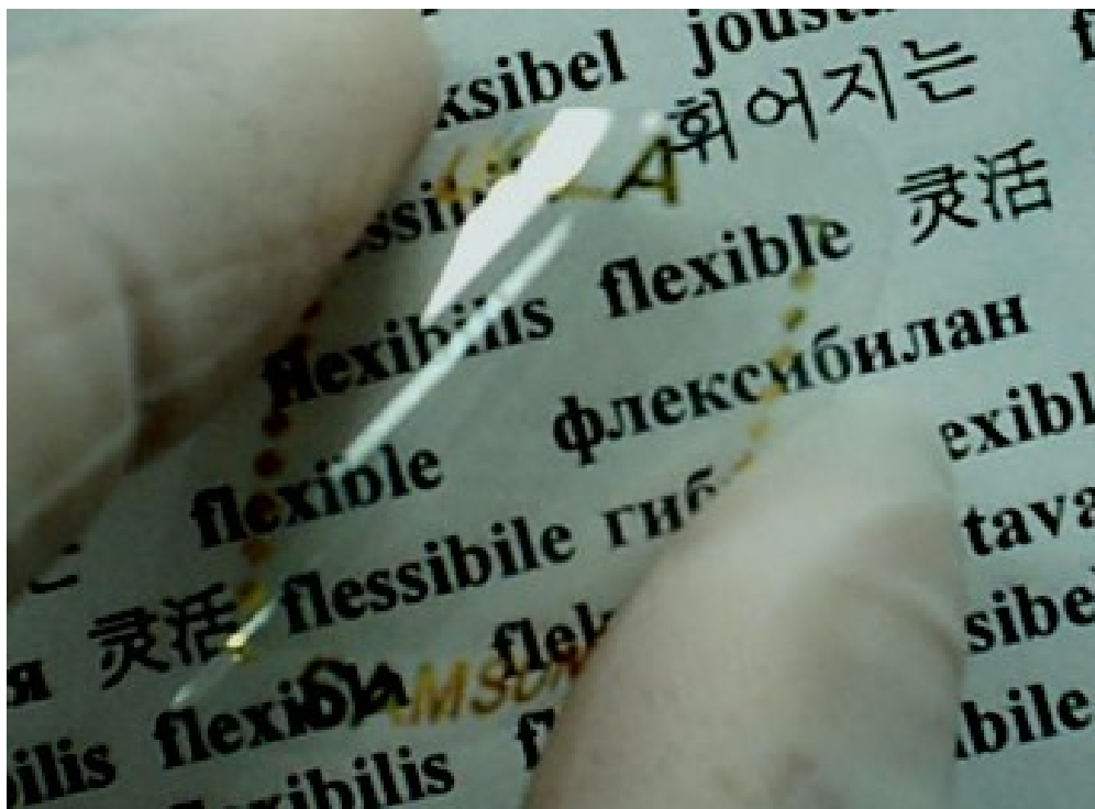
Figure 3.6 Photographs of the large scale transparent-flexible FTM array fabricated on PEN substrate. FTM cell is transparent enough to see objects through it without image distortion.
