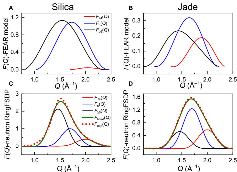
**Fig. 5. Deconvolution of the FSDP into contributions from different ring size groups.** The grouped  $F_n(Q)$ -FSDP contributions computed from FEAR-based glass structure match with  $F_n(Q)$  deconvoluted by RingFSDP method for (A and C) silica and (B and D) Jade glasses. For clarity, in (A) and (B), a linear background is subtracted from the computed structure factors to better isolate the FSDP peak. (C) and (D) The decomposition of the experimental FSDP following the RingFSDP approach.
