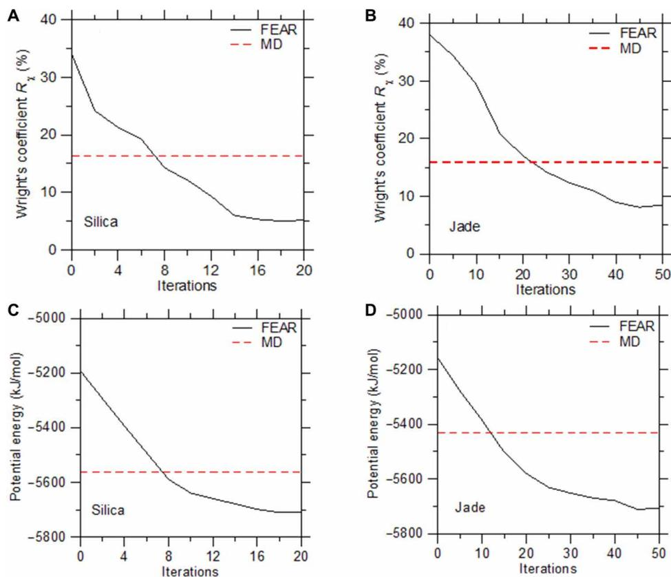
**Fig. 8. Comparison of the Wright's coefficient,  $R_x$  (A and B) and molar potential energy (C and D) by FEAR and MD simulation.** Results are presented for the (A and C) silica and (B and D) Jade glasses. These data are compared with those obtained by MD simulations (shown as horizontal dashed lines) using the melt-quench approach (using a cooling rate of 1 K/ps).
