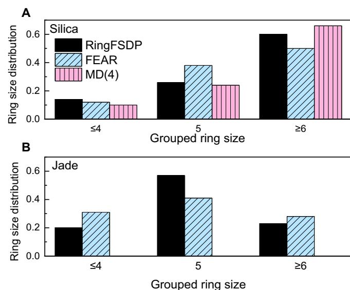
**Fig. 7. Ring size distribution comparison between the experimental RingFSDP and FEAR/MD simulation analysis.** (A) silica and (B) Jade glasses. The good match between experiment and modeling validates the RingFSDP method.
