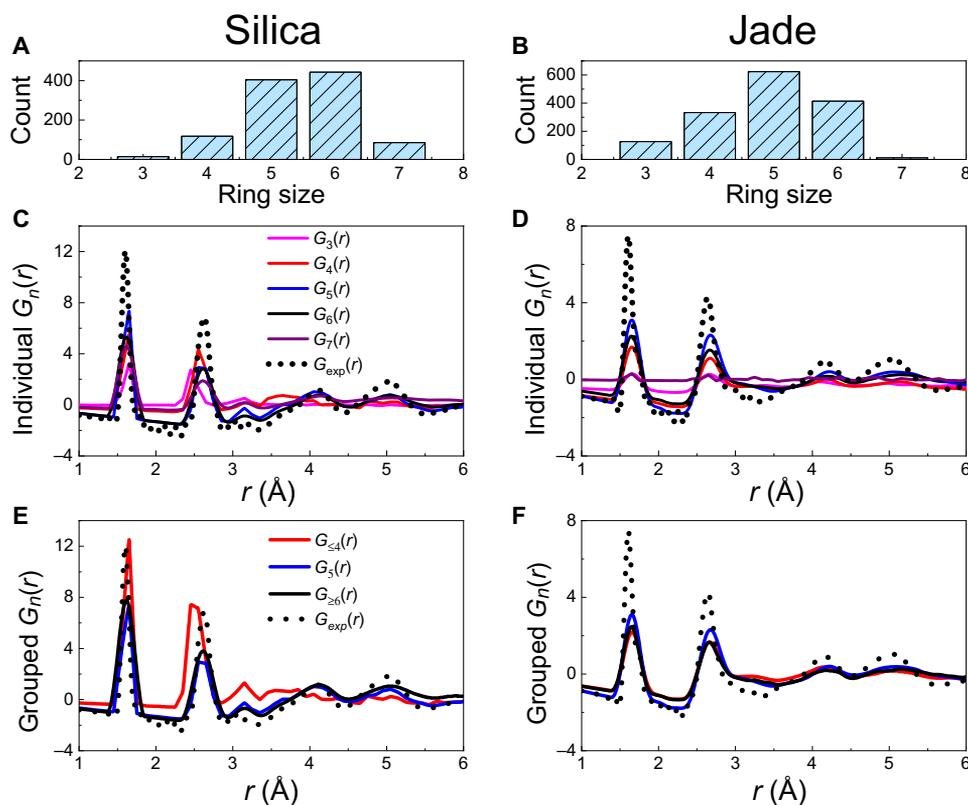
**Fig. 3. Guttman's ring size distribution.** (A and B), reduced PDF  $G_n(r)$  of individual (C and D), and grouped (E and F) rings computed from the FEAR simulations. Note that the individual PDFs are associated with fixed ring sizes  $n$  (with  $n = 3$  to 7), while grouped PDFs are associated with groups of rings (i.e.,  $\leq 4$ -, 5-, and  $\geq 6$ -membered rings, as defined in the RingFSDP method). They are compared to the experimental neutron data (black dot curve).
