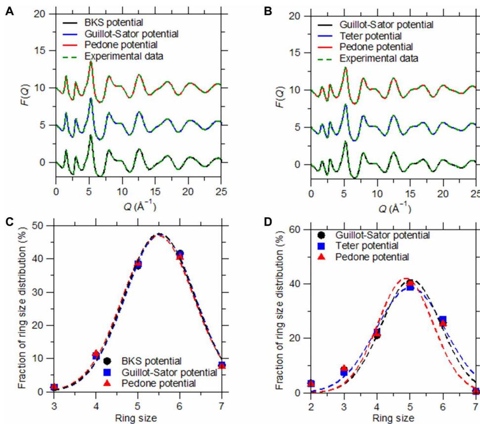
**Fig. 9. Comparison of the structure factor.**  $F(Q)$  (A and B) and ring size distribution (C and D) computed by FEAR while using different interatomic potentials. Results are presented for the (A and C) silica and (B and D) Jade glasses.
