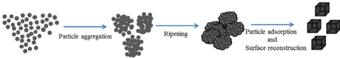
Figure 7 Growth mechanism of barium titanate through the composite-hydroxide-mediated synthesis method [7].
